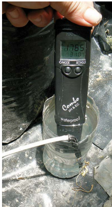
Fig. 9.2. EC meter for measuring the concentration of nutrient solutions.
