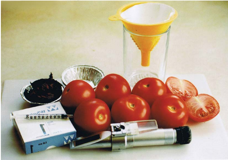
Fig. 13.2. Brix testing is a common compositional quality assessment.
