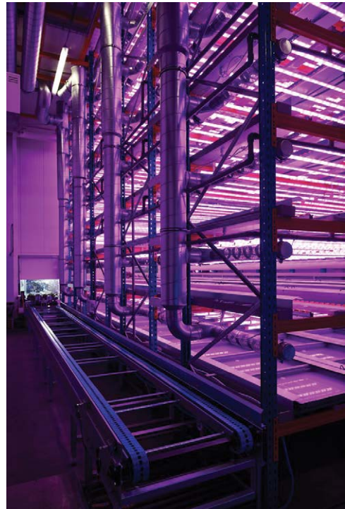
Fig. 12.2. Use of conveyor systems maximizes space in an automated plant factory. (Image courtesy of Urban Crop Solutions, https://urbancropsolutions.com , accessed 11 September 2020.)
