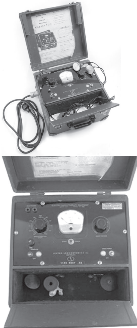
Figure 10-4: ECT machine; overview with cables (top), close-up of the operating board (bottom). Manufacturer: Lektra Laboratories Inc., 1960. Source: Courtesy of the Museum of Health Care at Kingston.
