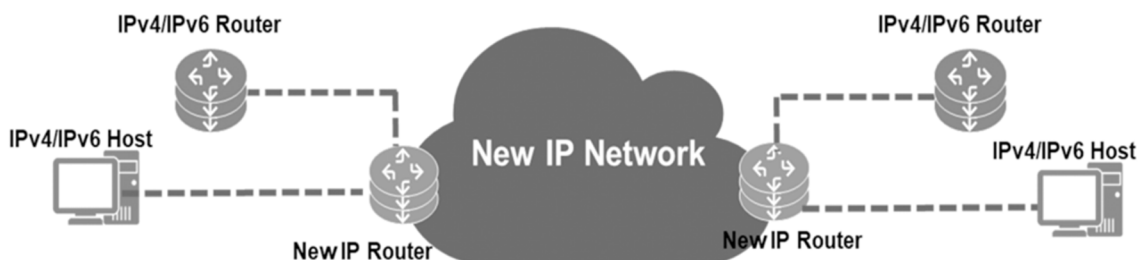
Figure 11. Legacy host/routers interaction with New IP island
