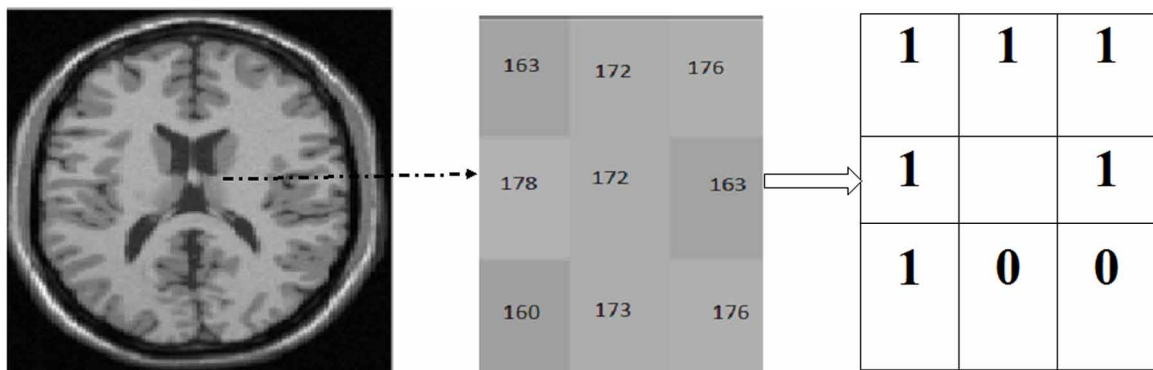
Figure 1. LBP model for a 3x3 window taken from the T1 MRI white matter region
