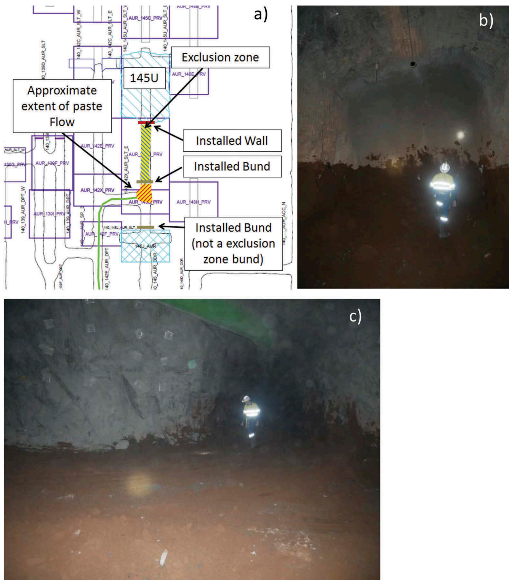
Figure 9. Paste 145U overfill showing a) level plan with approximation of location of bunds, b) paste staining at the shotcrete wall location, and c) paste staining along the drive.
