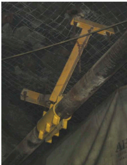
Figure 4. Example of anchor support used at Eleonore.
