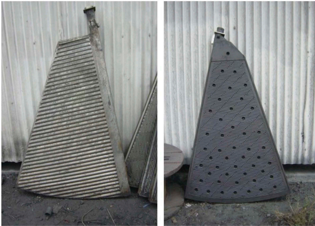
Figure 4. Old and heavy (40 kg) filter segments (12 segments per disc).
