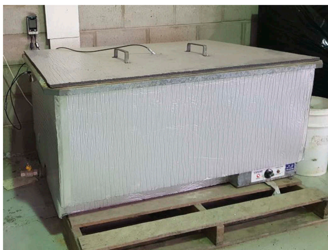
Figure 9. Photograph of insulated curing chamber.
