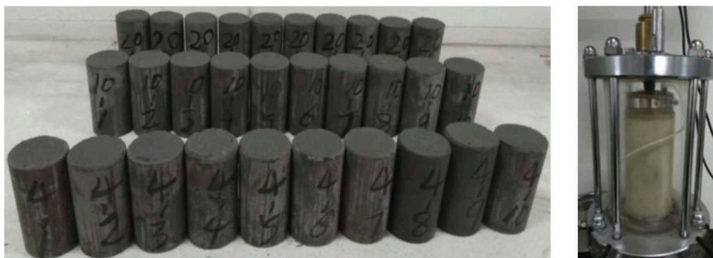
Figure 5. Casted cylindrical backfill samples for triaxial compressive tests.
