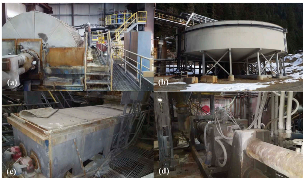
Figure 3. Photos of existing paste plant, (a) view of disc filter (left) and cyclones (right); (b) view of thickener adjacent to paste plant; (c) continuous mixer; (d) positive displacement pumps.
