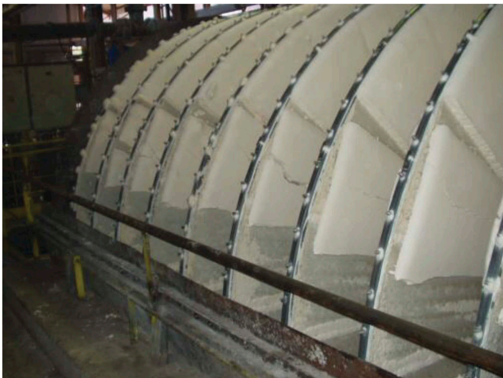
Figure 3. Complete cake discharge of a type A disc filter after revamping with “large package” modifications.
