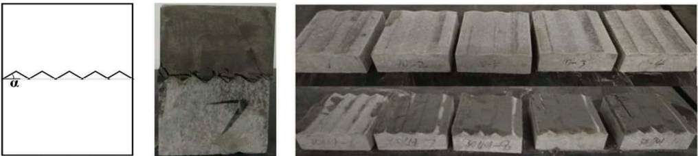
Figure 3. Nonplanar interface with different roughness and typical shear tested samples.
