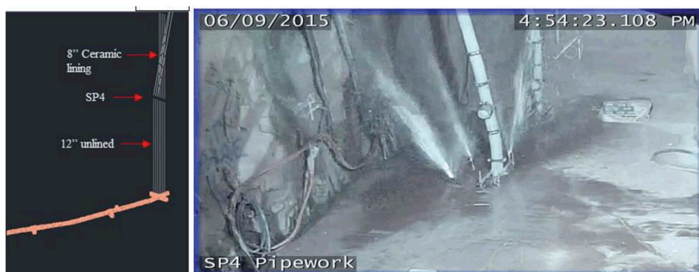
Figure 15. Surface borehole sketch and photograph showing blowback at mid borehole level.
