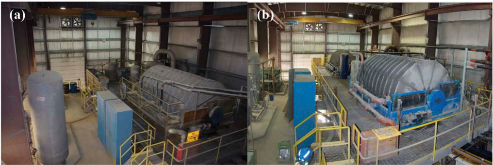
Figure 6. Comparison between (a) Existing filter level layout and (b) Retrofit filter level layout.
