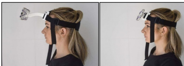
Figure 3. MOVE-IT long arm head mount device on left, short arm head mount device on right.
