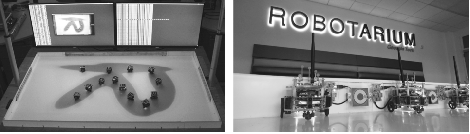
Figure 9.4: Two versions of the Robotarium platform. Left: A coverage control algorithm is executed on an early prototype version of the Robotarium using 13 “GRITSBot” robots [338]. The desired density function is projected onto the testbed arena in the shape of the letter R. Right: The Robotarium testbed with the newer “GRITSBot X” robots [431], charging at the inductive charging stations surrounding the Robotarium. Note the nonsymmetrical markers mounted on top of the GRITSBot X robots used by the motion captioning system to uniquely identify the robots. Source: Fig. 1 in Pickem et al. (2017).
