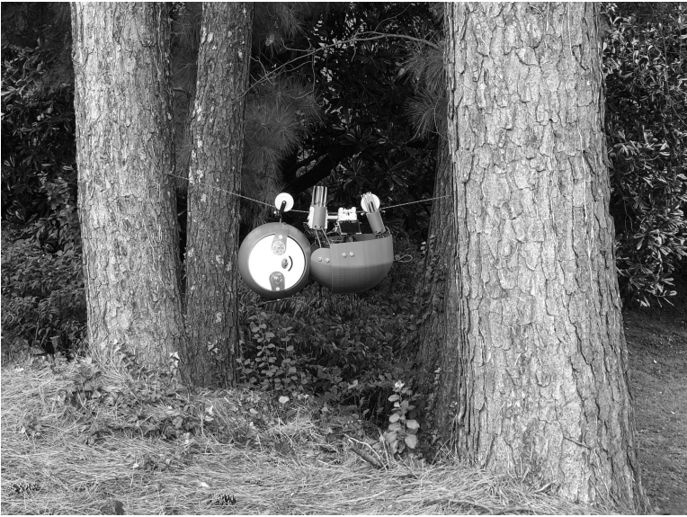
Figure 1.2: The SlothBot—a slow and energy-aware robot developed to perform environmental monitoring tasks—traverses a cable suspended between trees on Georgia Institute of Technology’s campus.
