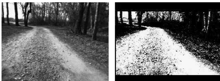
Figure 3.1: The robot from Figure 1.4 is learning, over time, to predict “terrain preferability” by interacting with the environment (literally, by driving into things). Left: Camera image. Right: Classified cost of preferable terrain, where lighter terrains are classified as more preferable from an ease-of-navigation vantage point.
