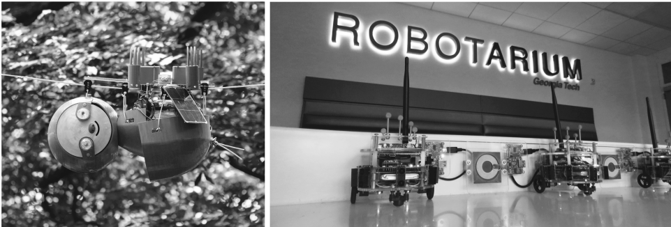
Figure 7.10: The SlothBot (Left) and Robotarium (Right) constitute canonical instantiations of the robot ecology concept, designed for long-duration environmental monitoring and autonomy-on-demand, respectively.
