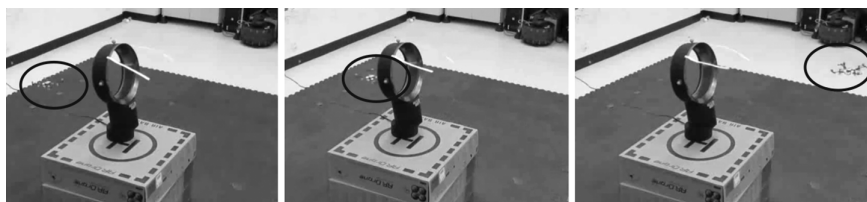
Figure 4.12: By incrementally probing the airflow around a fan, the quadrotor learns how to fly through the blade-less fan in a safe manner. Additionally, a GP model is produced as part of this process, describing the effect the fan has on the quadrotor dynamics.
