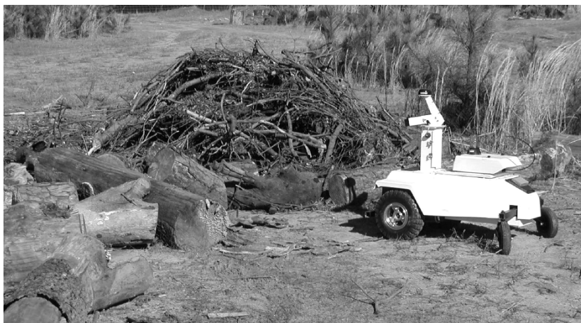
Figure 1.4: Based on an object's texture and color properties, a robot must learn which objects in the environment can be traversed and which cannot.
