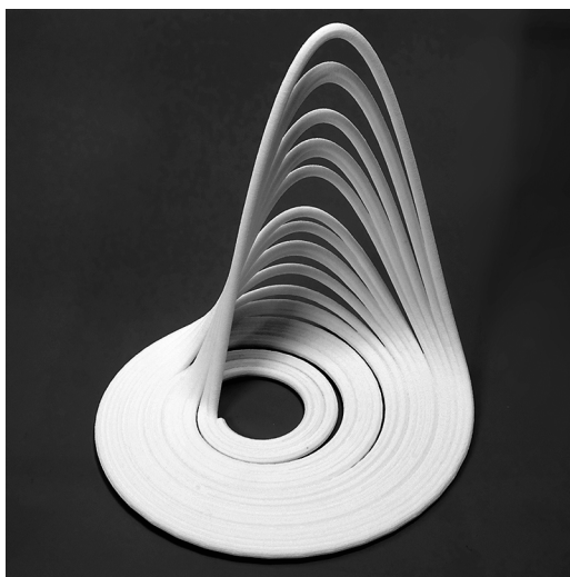
FIGURE 2. The Rössler chaotic attractor in Equation (5), modeled in MATLAB and OpenSCAD and 3D printed in selective laser sintering (SLS) nylon. Photo credit: Edmund Harriss. See also color insert.
