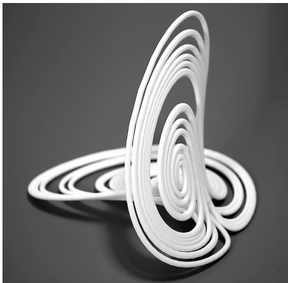
FIGURE 4. The Rucklidge chaotic attractor in Equation (10), modeled in MATLAB and OpenSCAD and 3D printed in SLS nylon. Photo credit: Edmund Harriss. See also color insert.
