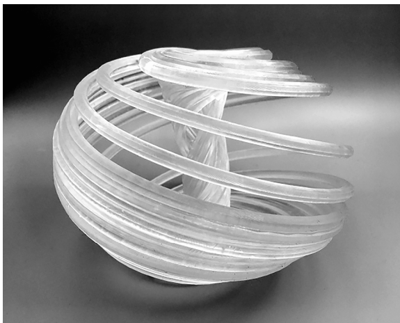
FIGURE 6. The Langford chaotic attractor in Equation (8), modeled in MATLAB and OpenSCAD and 3D printed in stereolithography (SLA) resin. See also color insert.
