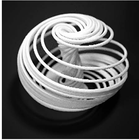
FIGURE 21. The Langford chaotic attractor in Equation (8). Modeled in MATLAB and OpenSCAD and 3D printed in SLS nylon. Photo credit: Edmund Harriss. See also color insert.
