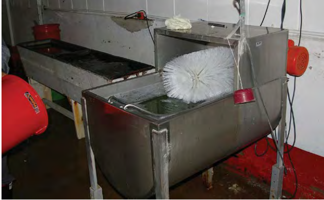
Fig. 8.10. Commercial bucket-washing equipment is necessary to clean the large number of buckets needed each day. (Photo: J. Dole.)
