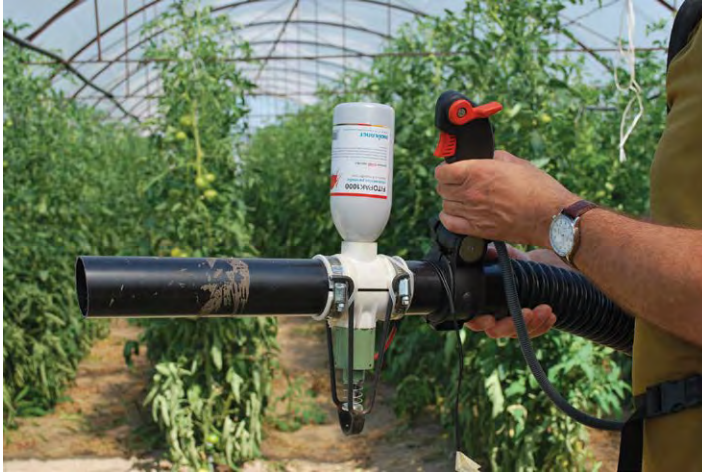
Fig. 7.8. A mechanical air blower for the application of predatory mites. (From Lanzoni et al. , 2017.)
