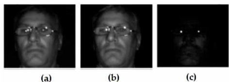
Figure 1. The driver's pupil: (a) first image; (b) second image from another IR sensor; (c) difference image
