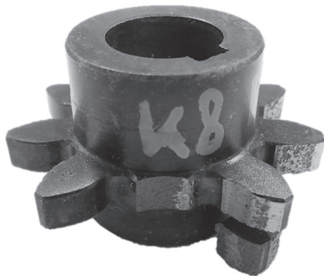
Figure 6.5: Typical fatigue fracture of a gear tooth (test gear K08)
