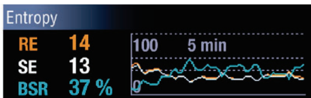
Fig. 9-6. The E-Entropy monitor displays two numbers: state entropy (SE) and response entropy (RE), with higher frequency EMG activity being included in the latter. Reproduced with permission ( www.clinicalview.gehealthcare.com ).
