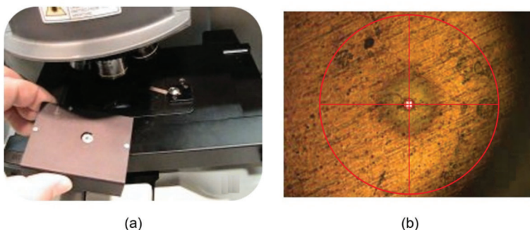
Figure 3-3. The alignment and calibration tool to be placed on the microscope stage (a), and the bright pinhole of the tool in the optical focus centred on the microscope eyepiece crosshair (b).
