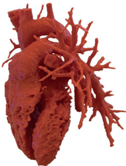
Fig. 5.4: Fused deposition modeling approach allows labs to create personalized models of congenital heart diseases with approximately 24-h turnaround time from image acquisition. This fabrication technique was satisfactory here, as models are used only for visualization and not for simulation. The model in this picture was delivered to cardiologists from University Children's Hospital of Kraków.
