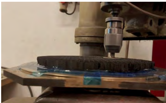
Figure 4.24: Honeycomb machining to obtain a flat surface.
