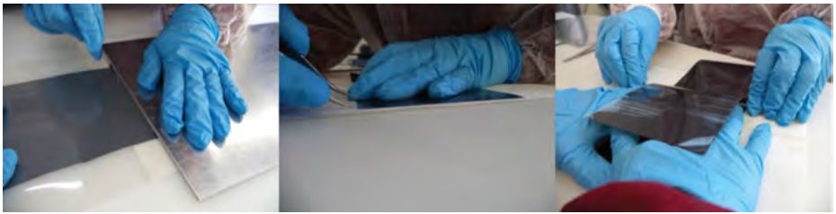
Figure 4.9: Procedure used for cutting and removing the supporting film from the buckypaper.
