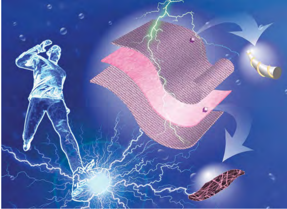
Figure 3.2: Sketch showing power generation from human movement using fiber-based piezoelectric generator. Reproduced from Refs. [23, 26] with permission from the Royal Society of Chemistry.
