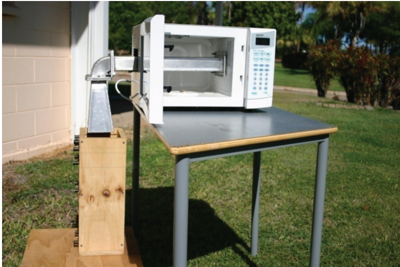
Figure 8.1: Prototype system, fed from the magnetron of a 800 W microwave oven (Source: Bebawi et al., 2007).
