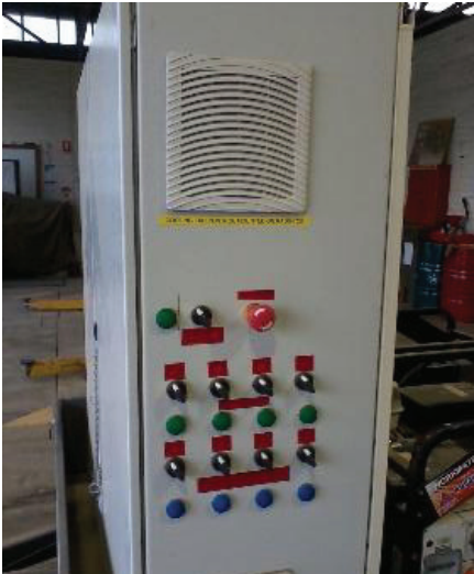
Figure 8.3: Prototype four by 2 kW microwave weed killer (above) with details of the control panel (below).
