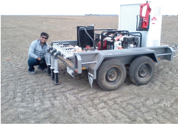
Figure 7.7: Trailer mounted four by 2 kW microwave weed killer.
