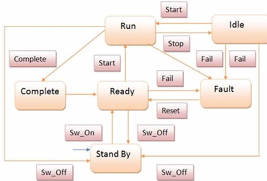
Figure 5. Appliance Finite State Machine
