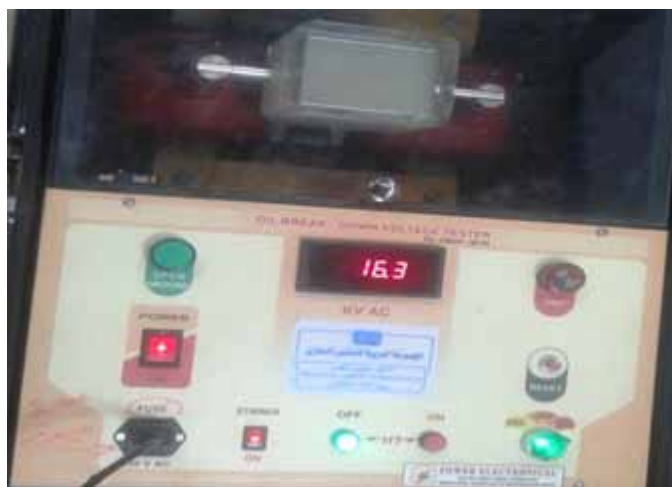
Figure 12. Motorized Oil Breakdown Voltage Lab-tester
