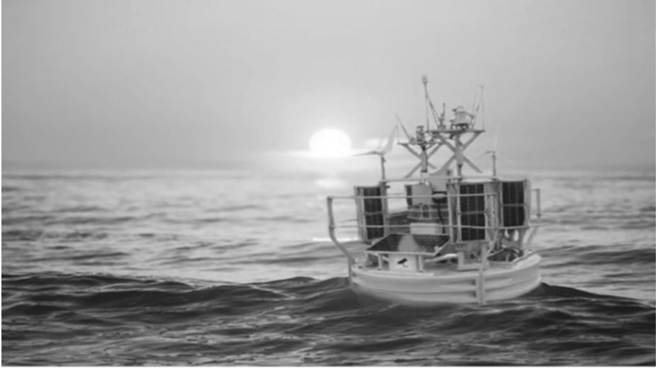
Figure 3.36: Blue Aspirations ZX300M Model Floating Lidar System. Source: Photo courtesy of Blue Aspirations.
