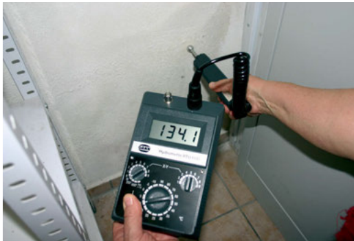
Fig. 7-45 Measuring the moisture, in the lower wall region about 134 digits, in the higher (drier) wall region about 107 digits.
