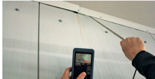
Fig. 7-40 Filling of the bead in the trapezoidal steel sheet without airtight seal, measurement of the natural air emission at the measuring point (here v = 0.20 \text{ m/s} ).
