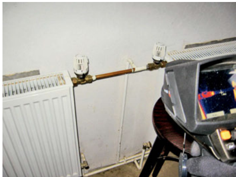
Fig. 2-10 Choosing a global emissivity doesn't represent the temperature correctly in this thermogram of a heating pipe due to the different real emissivity of the black- and white-coated pipe sections.
