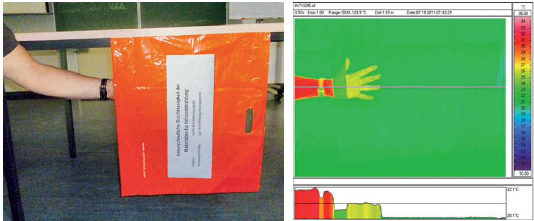
Fig. 2-19 Plastic films are often very transparent for infrared radiation; however, they are impervious for visible wavelengths.
