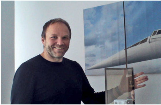
Fig. 2-17 Normal window glass is pretty much impervious to heat radiation; you can also see the thermographic camera mirrored in the image.
