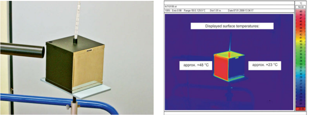
Fig. 2-9 Thermogram of a Leslie cube with a chosen global emissivity in order to illustrate the impact of different actual emissivity values of the surfaces. The surfaces of the cube have a steady temperature of about 48°C, but in the thermogram the temperature of the right side of the cube (polished metallic) is significantly lower than the actual temperature.
