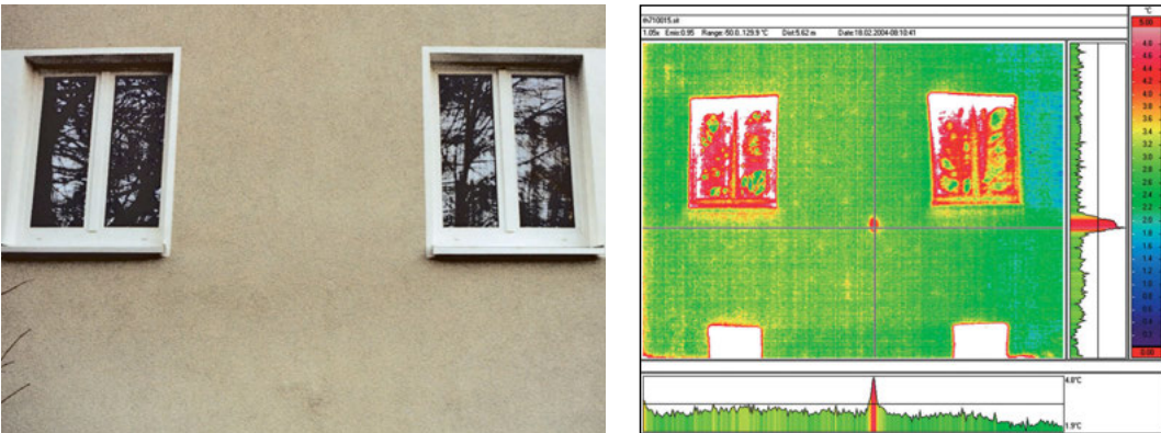
Fig.7-79 More detailed picture of the anomaly detected in Fig. 7-78: the elevated surface temperature \theta_{se} between the windows stands out against the rest of the facade (measured temperature: 4.4°C).
