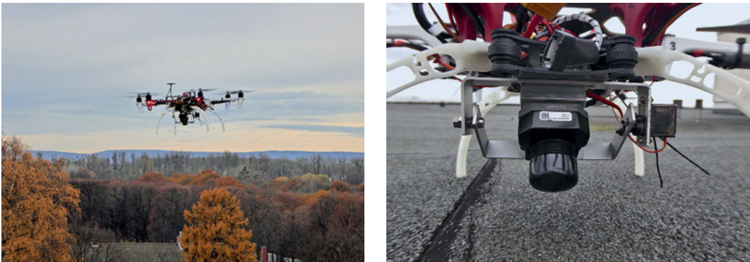
Fig. 7-50 Drone system (manufacturer DJI) with thermal camera Flir Tau2 (company Teax).
