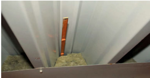
Fig. 7-40 Filling of the bead in the trapezoidal steel sheet without airtight seal, measurement of the natural air emission at the measuring point (here v = 0.20 \text{ m/s} ).
