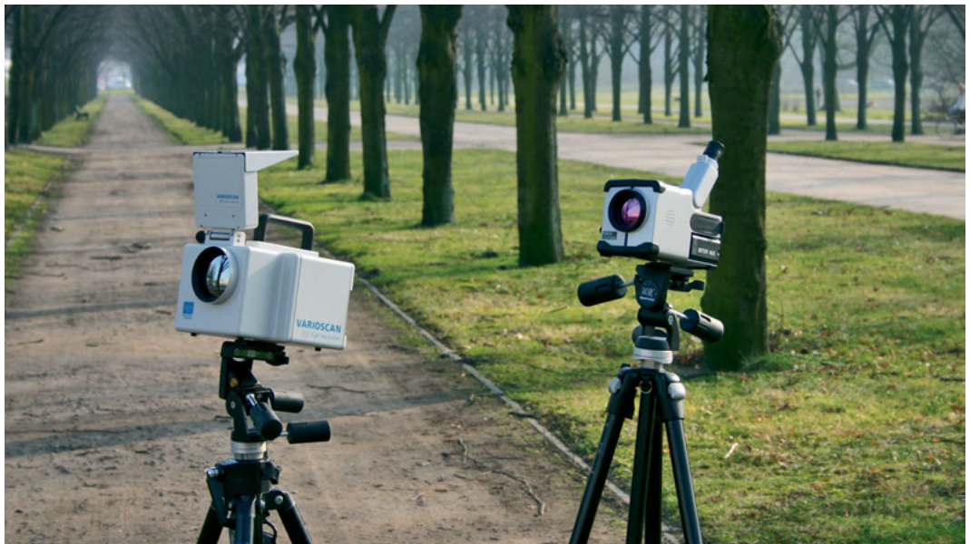
Fig. 3-9 Comparison measurement with thermography cameras: (left) scanning single-element camera equipped with a Stirling cooler; (right) uncooled micro-bolometer camera, with 320 × 240 pixels resolution (state-of-the-art in 2001).
