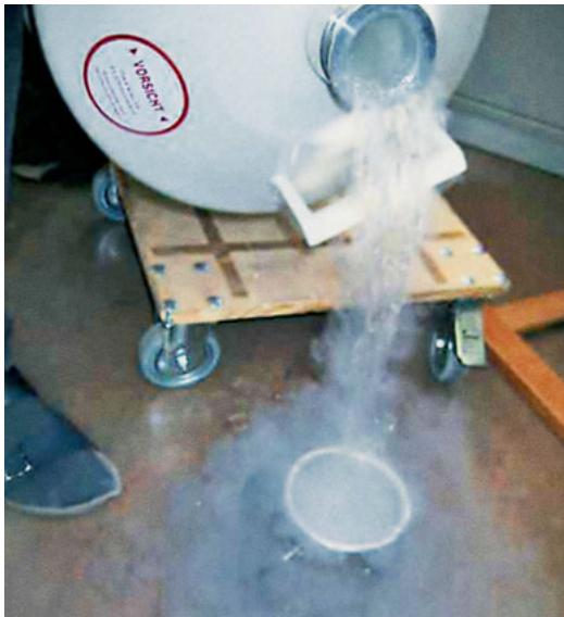
Fig. 3-2 Cooling with liquid nitrogen: A portable tank is filled with liquid nitrogen from a storage tank ( left ) and used to fill a thermography camera ( right ).
