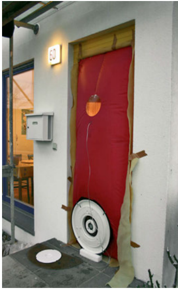
Fig. 7-29 Blower door in position (excess pressure measurement).
