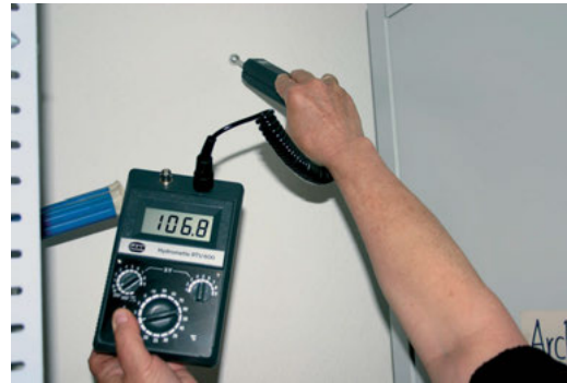
Fig. 7-45 Measuring the moisture, in the lower wall region about 134 digits, in the higher (drier) wall region about 107 digits.
