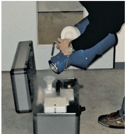
Fig. 3-2 Cooling with liquid nitrogen: A portable tank is filled with liquid nitrogen from a storage tank ( left ) and used to fill a thermography camera ( right ).
