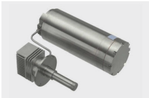
Fig. 3-3 Stirling cooler: linear-driven, split model (Image: Fa. AIM GmbH, Heilbronn 2003), 1.5 Watts refrigerating capacity (left: cold tip = cold finger, Ø 13.7 mm).
