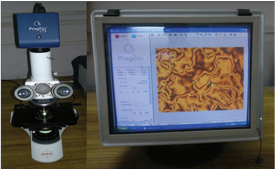
Figure 15.12: Complete setup for optical micrograph having polarizing optical microscope and optical texture on computer through interfacing software.
