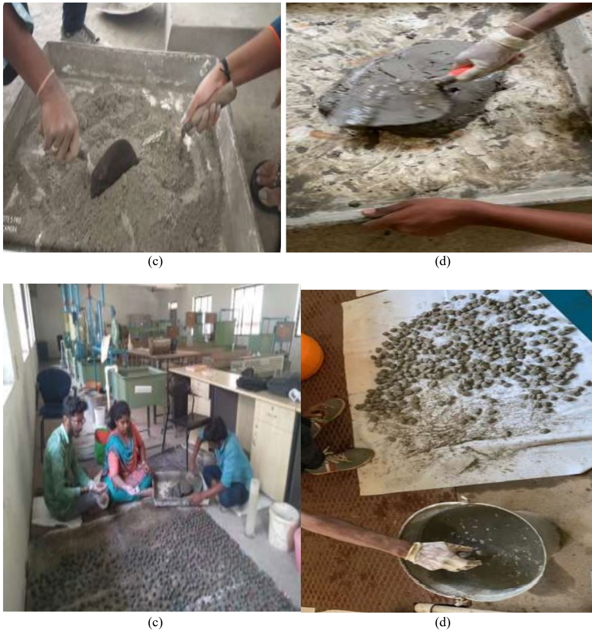
Fig. 1 Preparation of fly ash aggregate
