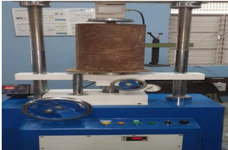
Figure 3. A shows the loading of clay soil through hydraulic jack with constantly increasing loading.
