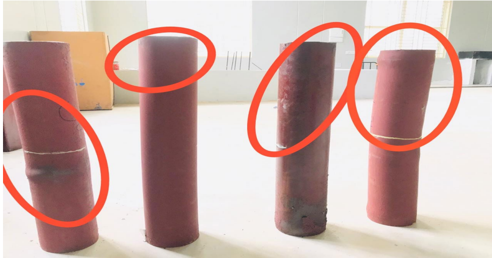
Fig. 4, Failure mode of Circular Specimen (600 mm Short Columns)
