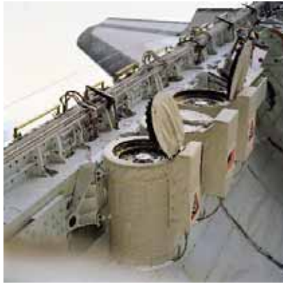
Fig. 5-2. Get Away Special Canisters inside the U.S. Space Shuttle cargo bay. Photograph NASA.
