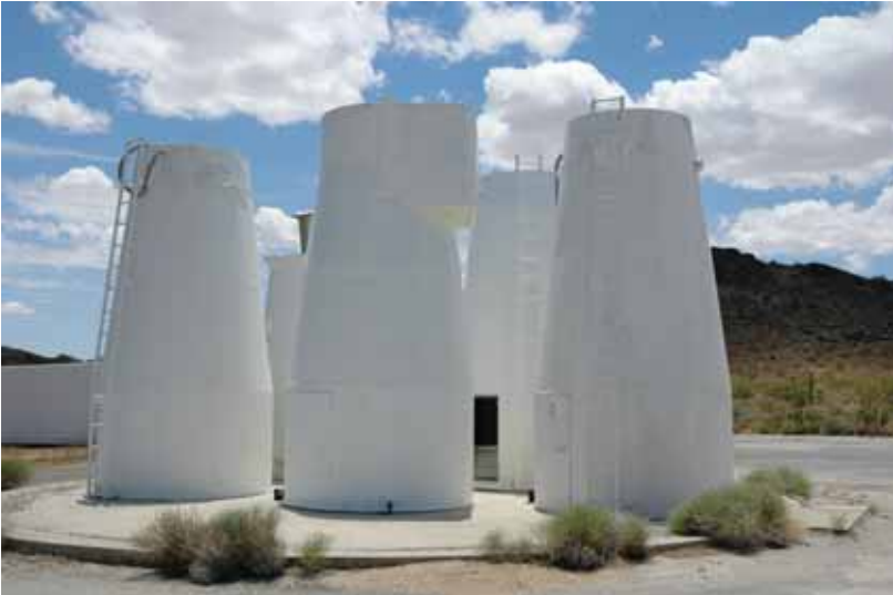
Fig. 5-3. Unused feed horns at NASA's Deep Space Network in Goldstone California. A feed horn goes in the middle of a radio antennae dish.
