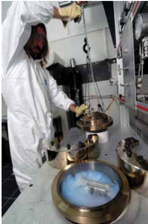
Fig. 2-1. The artist is opening the 20 litter high-temperature supercritical drying reactor after a continuous 48 hours run. The vessel was installed in Greece, September 2005, and all the aer( )sculptures have been created since then in it (photograph and copyright: Massimo Pizzocarò 2/2008).
