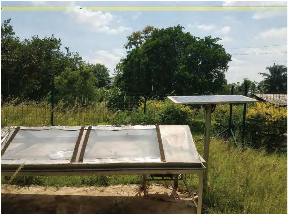
Fig. 3.3. Solar dryer fitted with a solar panel at the Kwame Nkrumah University of Science and Technology in Ghana.
