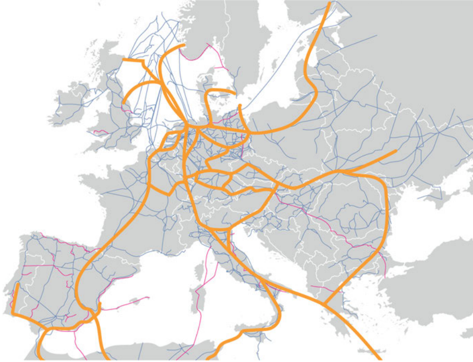
Fig. 23: Natural gas infrastructure in Europe (blue and red lines) and first outline for a hydrogen backbone infrastructure (orange lines). The main part of the hydrogen backbone infrastructure consists of re-used natural gas transport pipelines with new or retrofitted compressors. A new pipeline from the solar and wind resource areas in Greece needs to be realized as well as transport pipelines along the south coast of Portugal and Spain [33].
