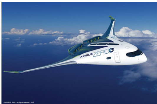
Fig. 28: The AirbusZEROe concept with hydrogen gas turbines and liquid hydrogen storage tanks [64].
