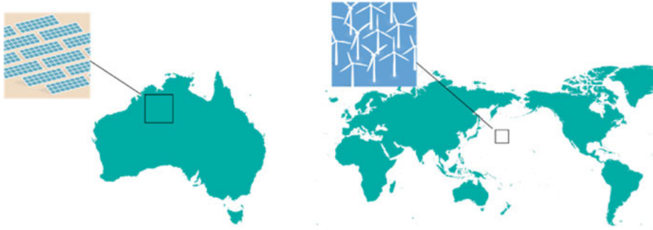
Fig. 3: Surface needed to meet global primary energy demand (155.000 TWh) by solar (10% of Australia) or wind (1.5% of Pacific Ocean) [1].
