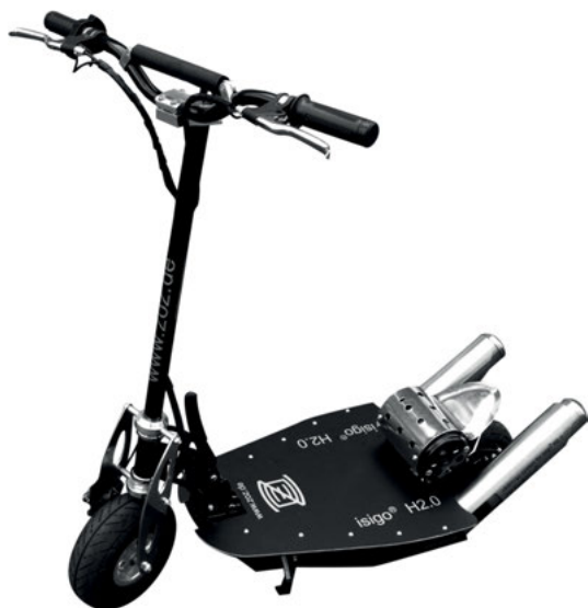
Fig. 17.10: Isigo ® H2.0 prototype with two H2Tank2Go ® cartridges.
