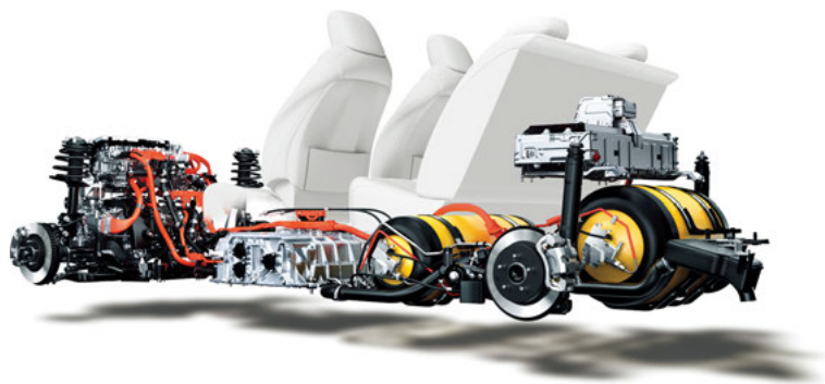
Fig. 3.25: Real installation of FC system in the vehicle (Toyota Mirai) (source: Toyota).
