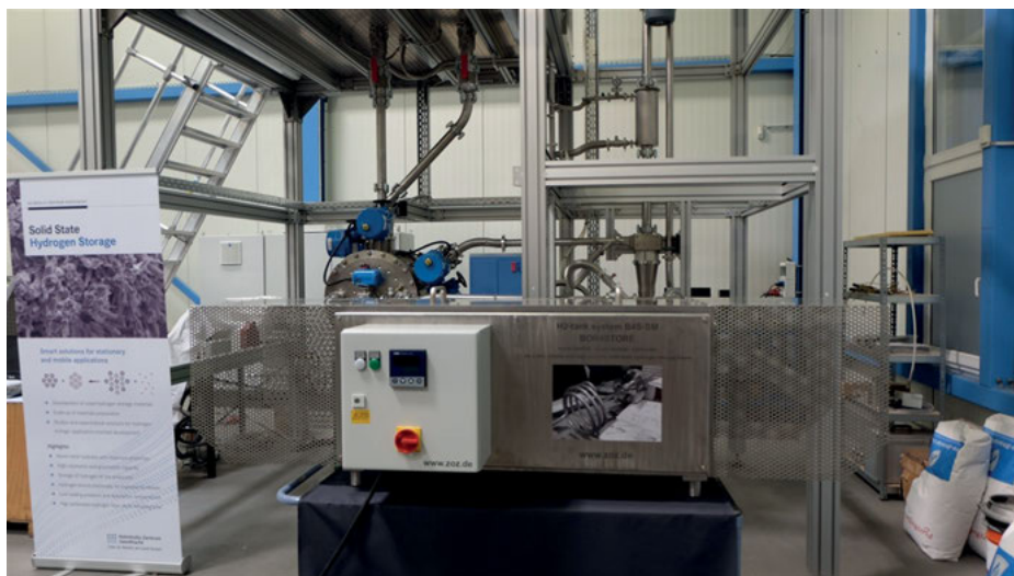
Fig. 17.7: H 2 tank system B4S-SM in the Helmholtz HZG – Hydrogen Technology Center in front of the Zoz-Simoloyer ® CM100-s2, a process plant for the production of complex metal hydrides.
