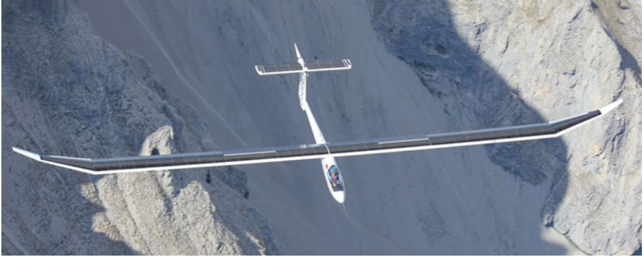
Fig. 17.12: Icaré 2 – record aircraft powered by solar power [25].
