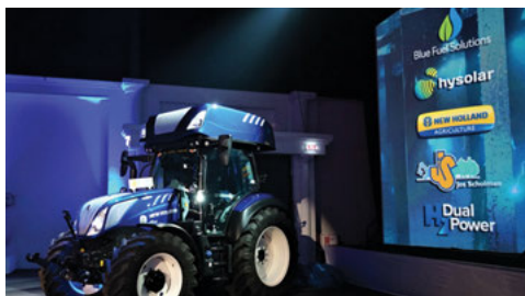
Fig. 29: H 2 Dual Fuel tractor, hydrogen can be blended in the diesel engine up to 80% [65].
