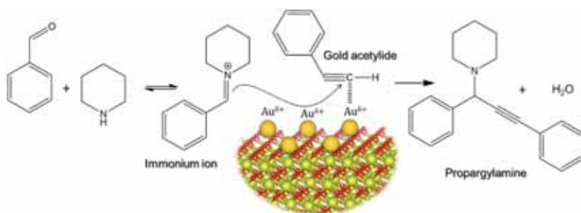
Figure 23 A^3 coupling reaction scheme over gold-supported catalyst
