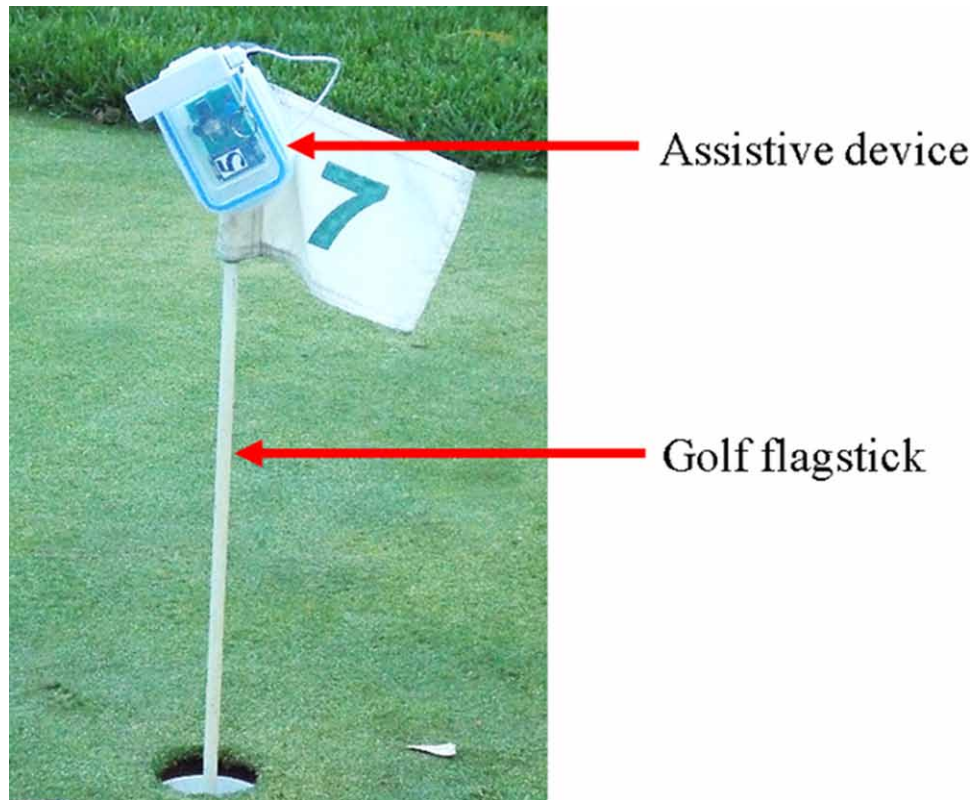
Figure 4. The assistive device attached to the top of the golf flagstick using Velcro straps.
