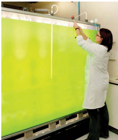
Fig. 15: A 100 L flat plate PBR as a pilot example for scaling up for future mass fermentation of cyanobacteria (coop. with KSD Co., Hattingen) [27].
