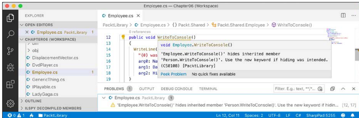
Figure 6.4: Hidden method warning
