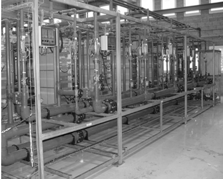
Fig. 12.7: Industrial implementation of the ED process in integrated zero-discharge technology of the company MEGA a.s. for processing sludge sulphate waters from uranium mining in the Czech Republic (photo: MEGA a.s.).
