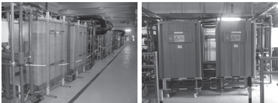
Fig. 7.33: Membrane stack casing options – on the left EDR-III by MEGA a.s., on the right EDR 2020 by GE Water & Process Technologies (now Suez Water Technologies & Solutions) (photo MEGA a.s.).
