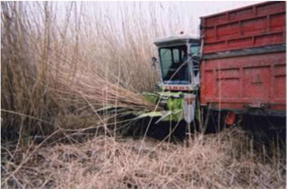
Figure 3.23: The three-row CLAAS Jaquar 690cl mower-fodder-loader combining machine.
