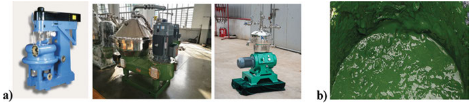
Figure 4.10: a) Separator centrifuges; b) Algal concentrate.
