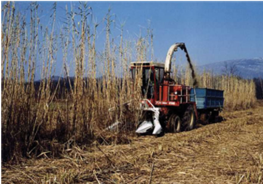
Figure 3.22: The three-row mower-fodder-loader combining machine – HESTON 7650 (Source: CETA).
