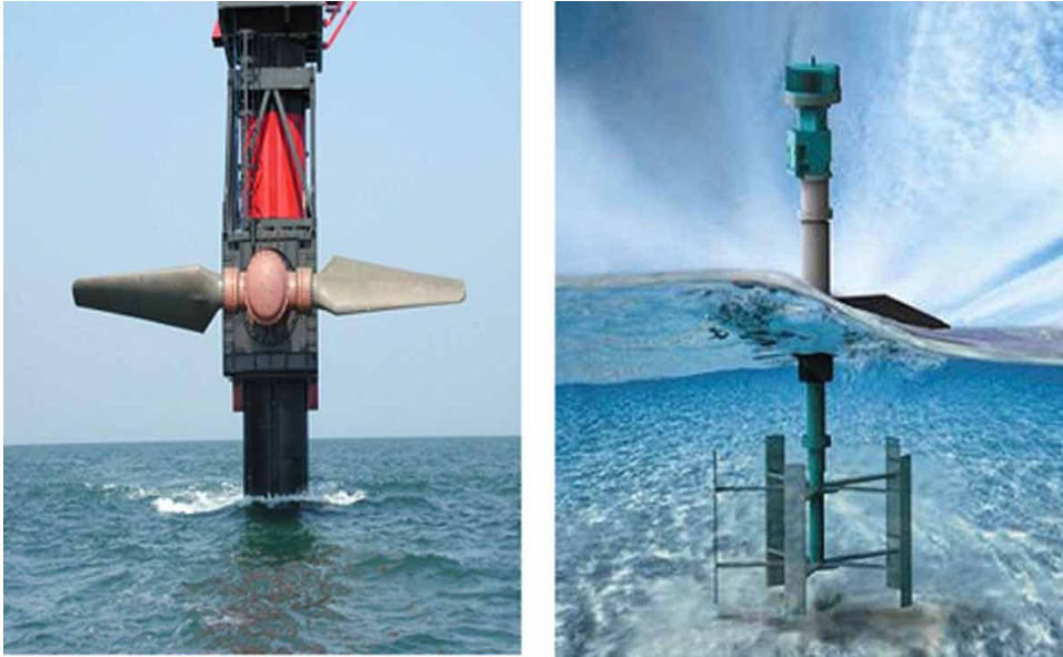
Figure 6. Tidal current / stream turbines (A) Horizontal-axis turbine (B) Vertical-axis turbine
