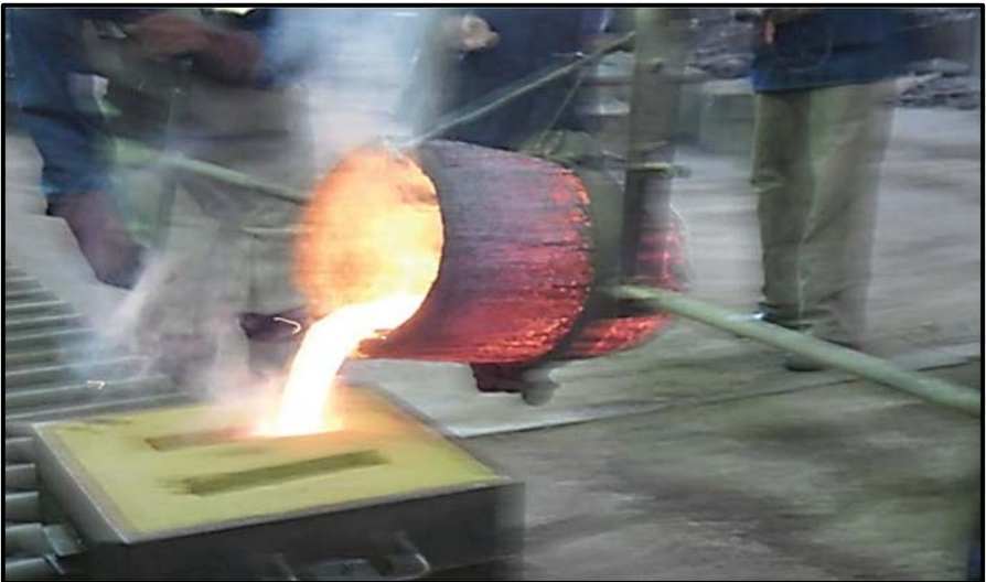
Fig 96: Casting Additional Experimental Samples. (Photo: the author)
