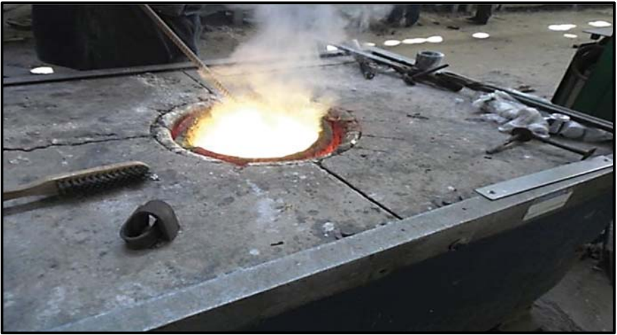
Fig 87: The Process of Taking out the Molten Metal. (Photo: the author)
