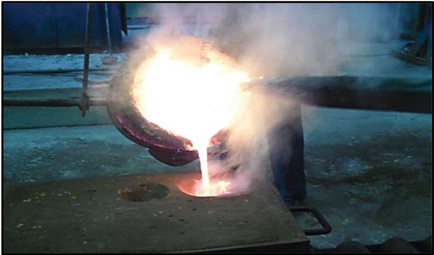
Fig 93: The Process of Casting Metal into Sand Molds. (Photo: the author)
