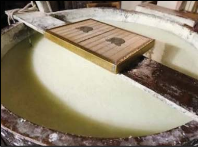
Fig 5: Addition of Watermark in Fabiano Factory. (Photo: Shutterstock Images).
