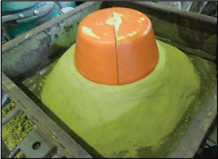
Fig 82: Sand Fingerprint of Wooden Ornic. (Photo: the author)
