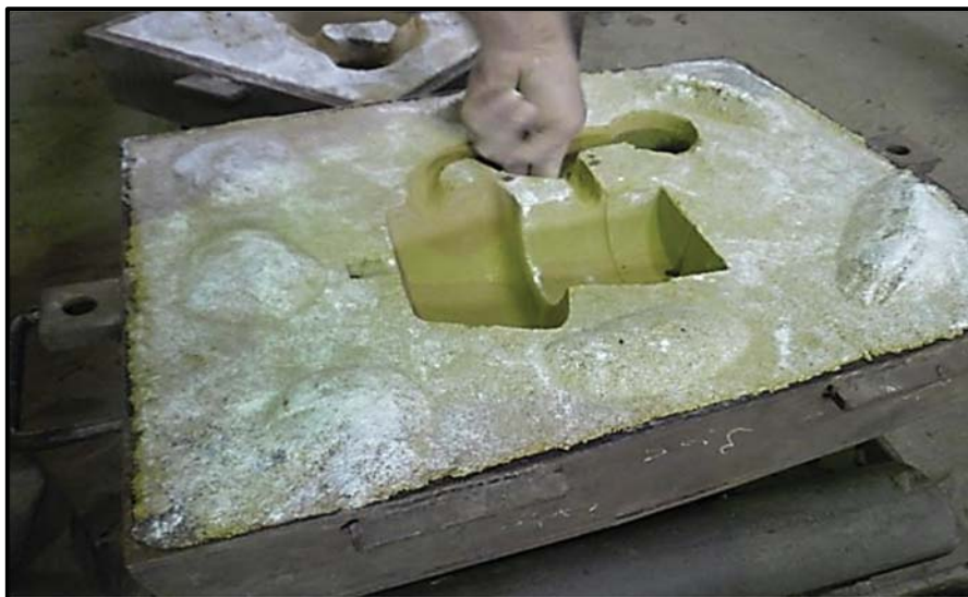
Fig 89: Preparing the Casting Channel in the Sand Mold. (Photo: the author)
