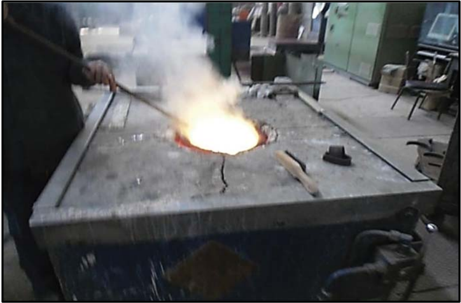
Fig 85: Melting Metal in a Melting Crucible. (Photo: the author)
