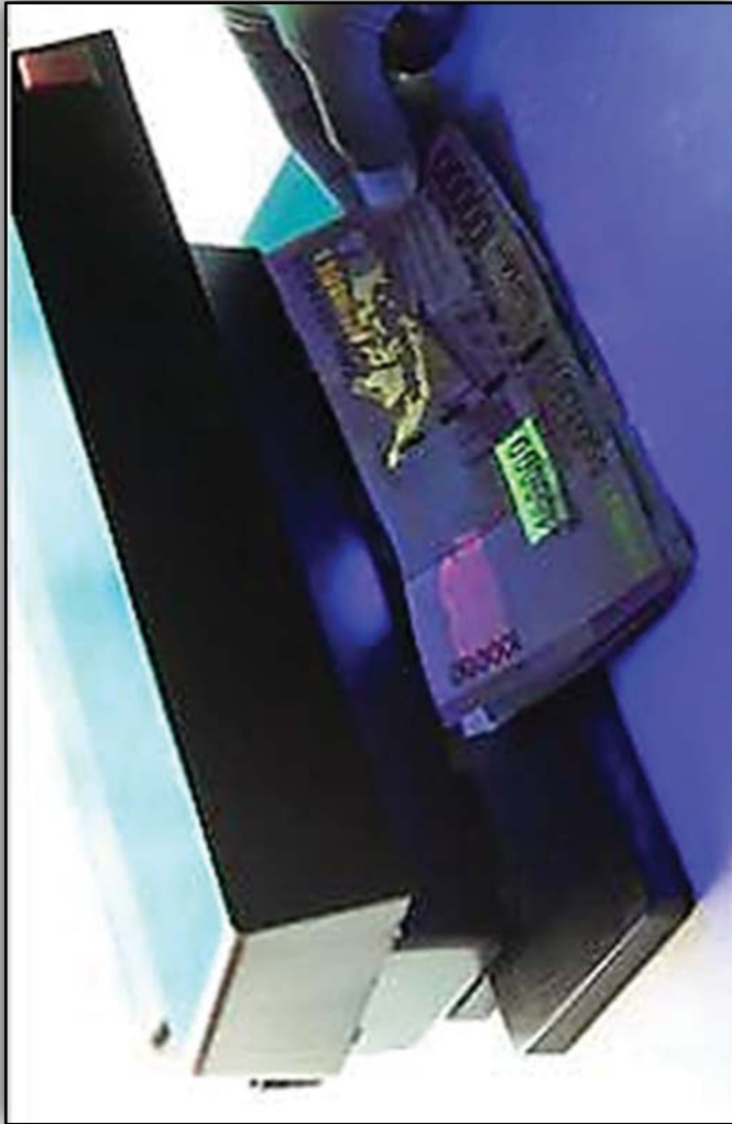
Fig 21: Examination of the Currency under Ultraviolet Rays. (Photo: Shutterstock Images).
