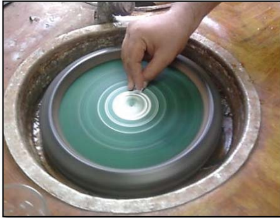
Fig 109: Process of Polishing Using Polishing Wheels. (Photo: the author)
