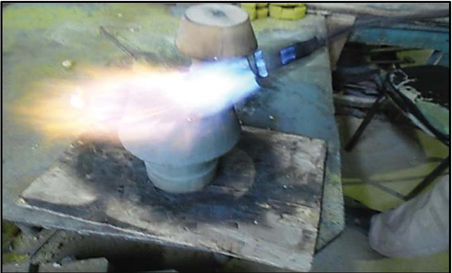
Fig 84: Drying Process of Sand Mold. (Photo: the author)
