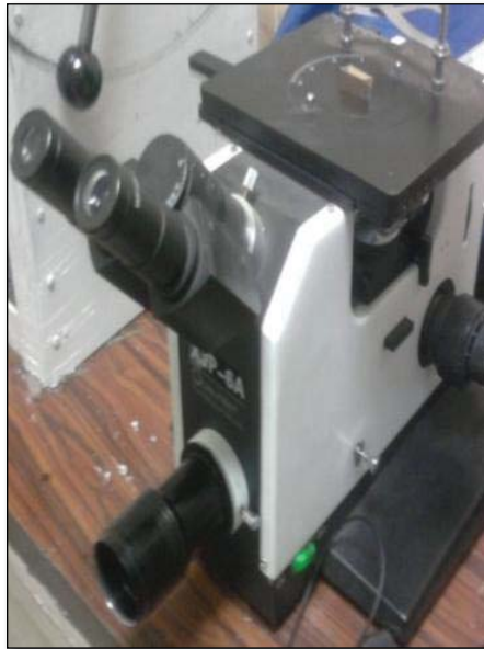
Fig 110: Copper Sample under a Metallographic Microscope. (Photo: the author)
