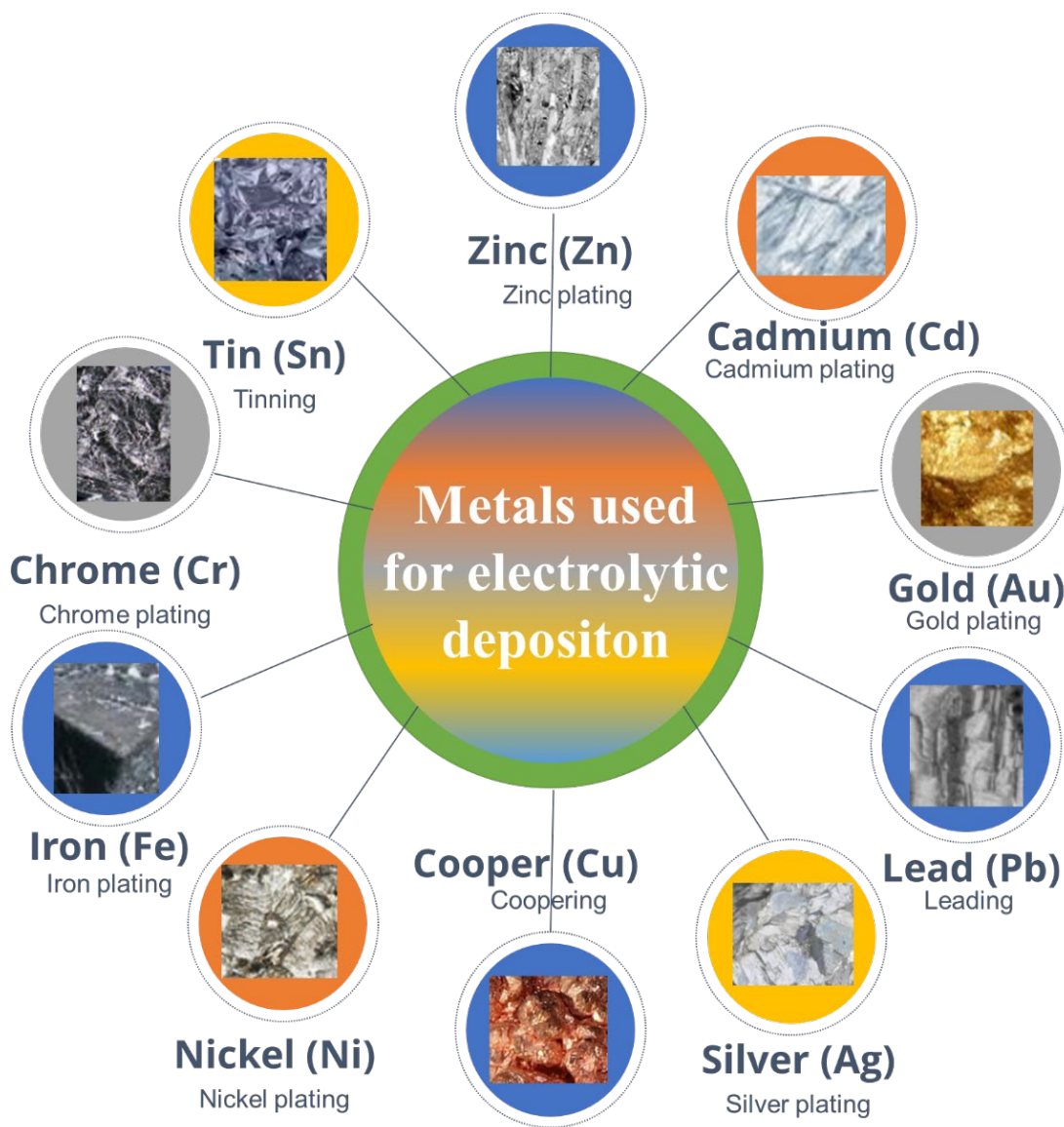
Figure 3.2. Metals used for electrolytic deposition.
