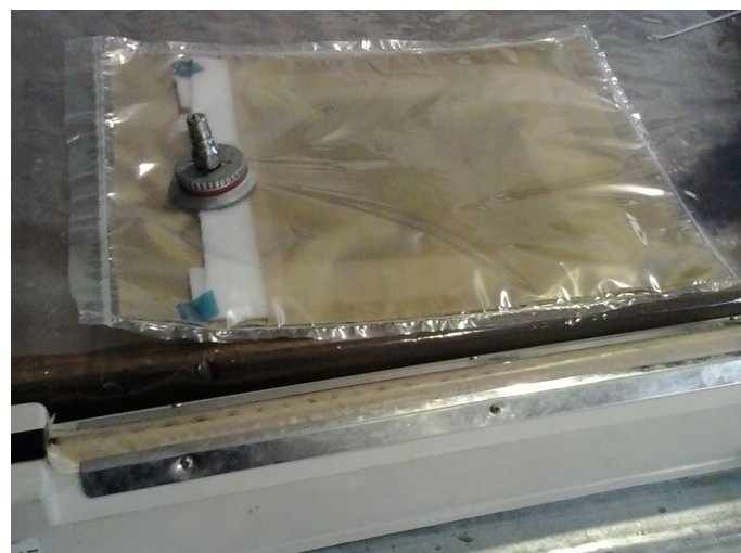
Figure 4.7. Sealing the bag and fixing the upper component of the previously inserted part.
