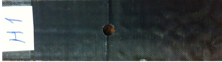
Figure 4.28. Carbon / epoxy hole laminate after test.
