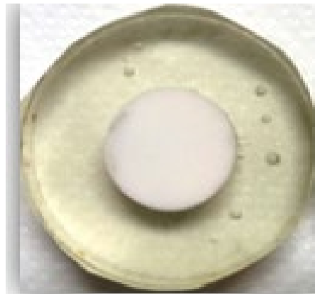
Figure 3.18. Sample embedded in epoxy resin, after surface polishing.
