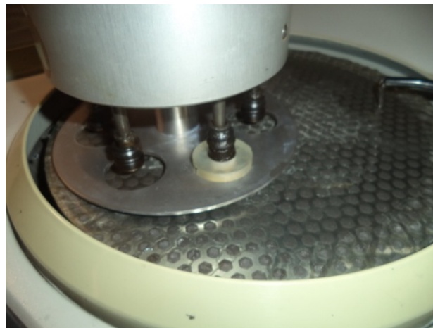
Figure 3.19. The first stage of sample polishing.
