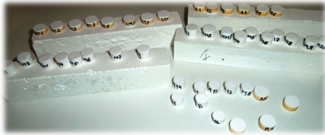
Figure 3.8. Sintered samples (the samples diameter is 10 mm).
