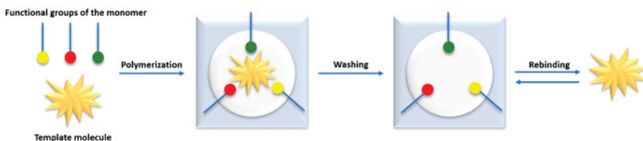
Figure 3.4: Schematic fabrication process of molecular imprinted polymers (MIPs). Reproduced with permission of MDPI [69].
