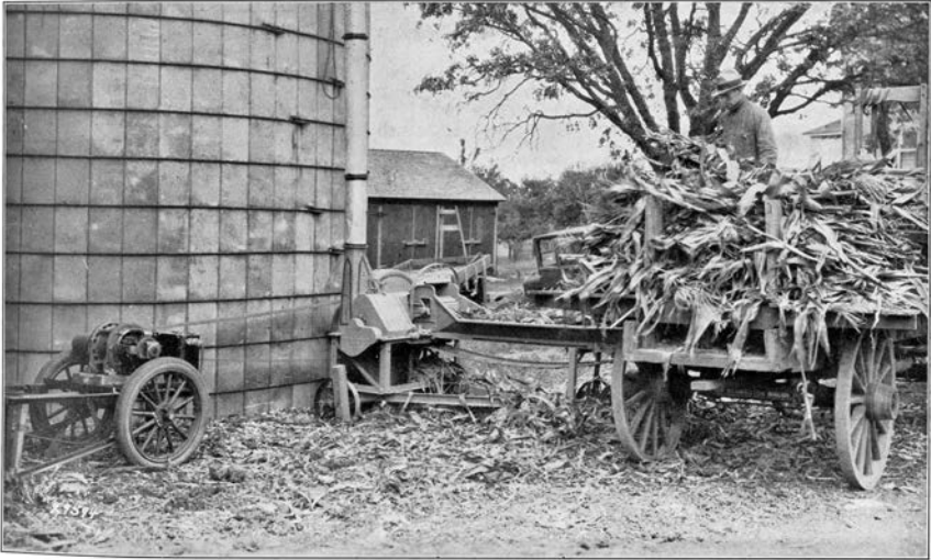
Fig. 9.8. An electric motor attached by belt to an ensilage cutter. Source: NELA, Electricity on the Farm and in Rural Communities , CREA Bulletin 4, no. 1 (30 January 1928): 55. Used with permission of the Edison Electric Institute.
