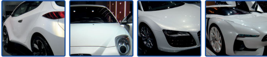
Figure 17.17: Pearl white stylings used both with a high gloss as well as with a matt clearcoat [160].
