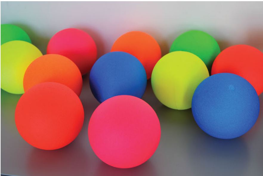
Figure 22.70: Luminescent colors have a special charm. Compared with normal chromatic colors, their colors are intensified by the conversion of UV light or visible light.
