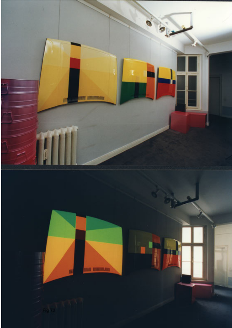
Figure 22.72: Hoods with absorption colors and afterglow colors under normal light conditions and in the dark.
