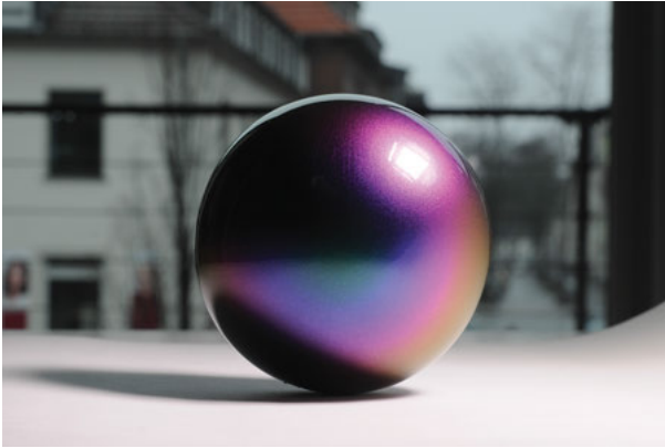
Figure 22.65: Color changes on the ball depend on the angle of illumination.
