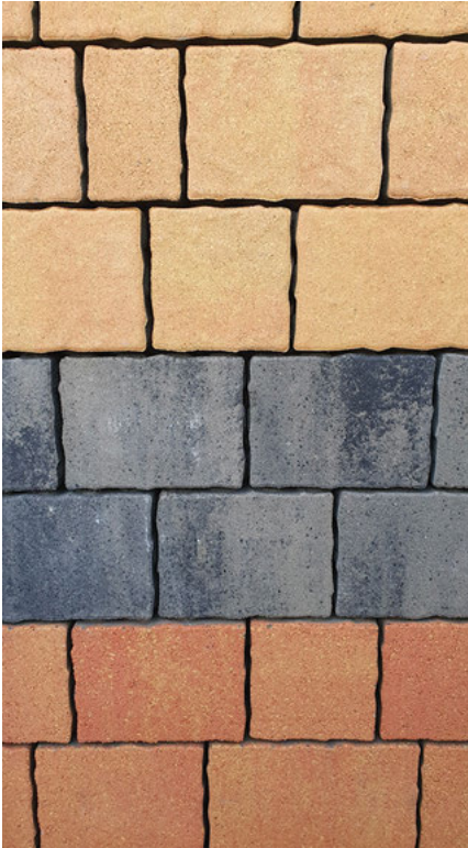
Figure 16.2: Concrete stones colored with different iron oxide pigments respectively pigment mixtures.
