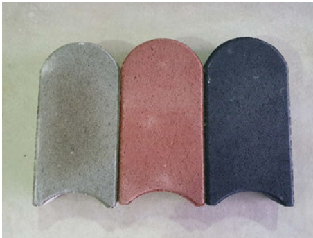
Figure 16.1: Concrete paving slabs, from left to right without pigmentation, pigmented with an iron oxide red pigment, pigmented with an iron oxide black pigment.
