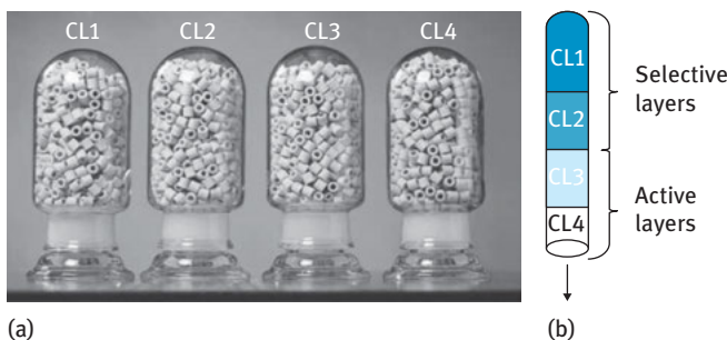
Figure 9.29: BASF O4-68 catalyst for o -xylene load of 80 g/N m 3 . From www.catalysis.basf.com/chemicals . (Copyright BASF SE).
