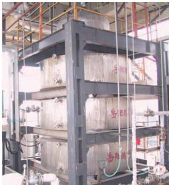
Figure 14.28: Magnetically stabilized bed reactor unit in caprolactam production with 100 kt/a capacity. From B. Zong, B. Sun, S. Cheng, X. Mu, K. Yang, J. Z. Zhao, X. Zhang, W. Wu, Green production technology of the monomer of Nylon-6: caprolactam, Engineering , 2017, 3, 379–384. http://dx.doi.org/10.1016/J.ENG.2017.03.003 . Open access.
