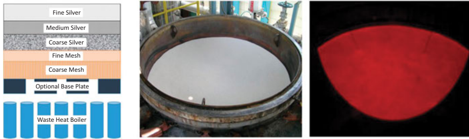
Figure 9.21: Left: Silver catalyst bed configuration; center: fresh bed; right: in operation. Reprinted with permission from G.J. Miller, M. Collins, Industrial production of formaldehyde using polycrystalline silver catalyst, Ind. Eng. Chem. Res. 2017, 56, 9247–9265. Copyright American Chemical Society.
