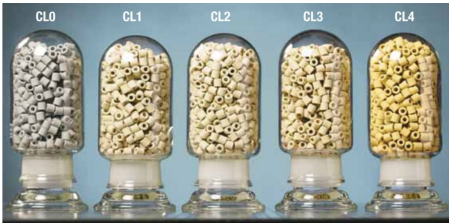
Figure 9.31: Five-zone BASF O4-88 catalyst for o -xylene load up to 100 \text{ g Nm}^{-3} (From https://catalysts.basf.com/public/files/literature-library/32012BF-9796-7152_BR_PUE_Catalysts_Anstcht.pdf ).
