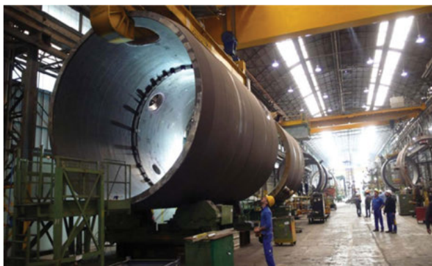
Figure 6.19: Eni Slurry moving bed hydrocracking technology: (a) scheme, (b) reactor (from https://www.eni.com/en_IT/attachments/innovazione-tecnologia/technological-answers/scheda-est-eng.pdf ).
