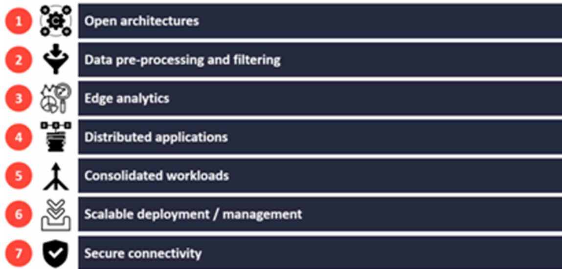
Figure 1. Seven characteristics of intelligent edge computing
