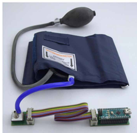
Figure 2. Measurement setup using an AMS 5915, Arduino Nano, the AMS 5915 Arduino Nano kit[4] and an inflatable cuff
