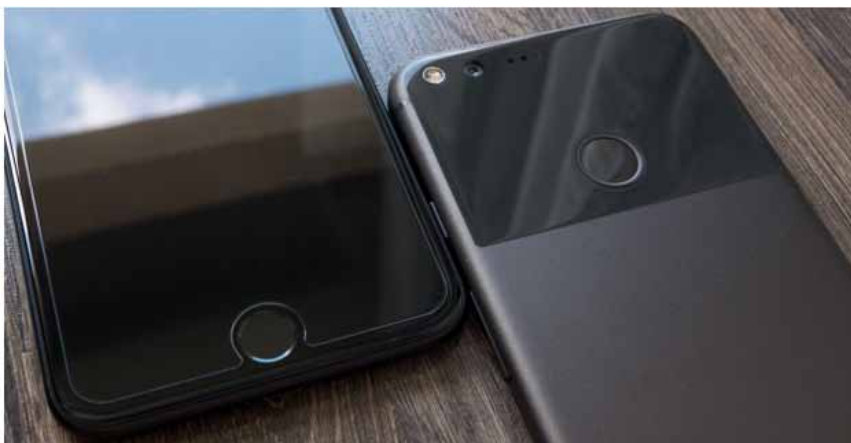
Figure 1. Shows a front fingerprint sensor along with a back fingerprint sensor (Patrick, 2017).
