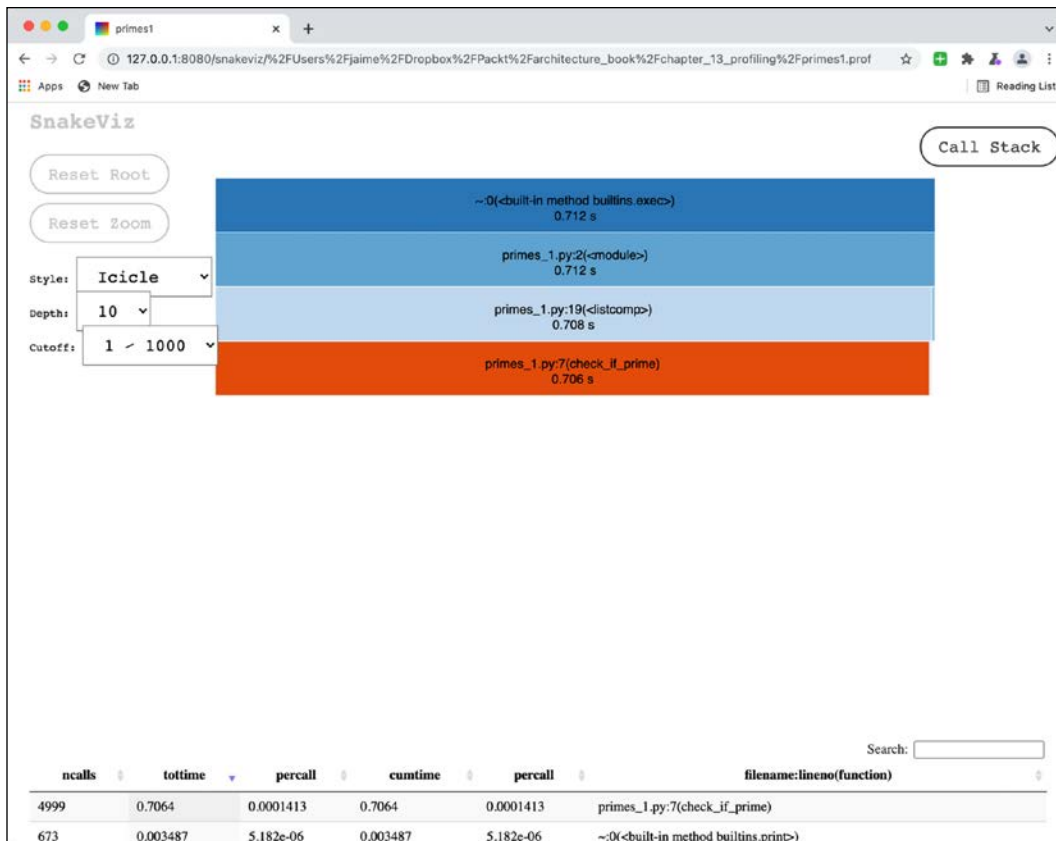
Figure 14.1: Graphical representation of the profiling information. The full page is too big to fit here and has been cropped purposefully to show some of the info.
