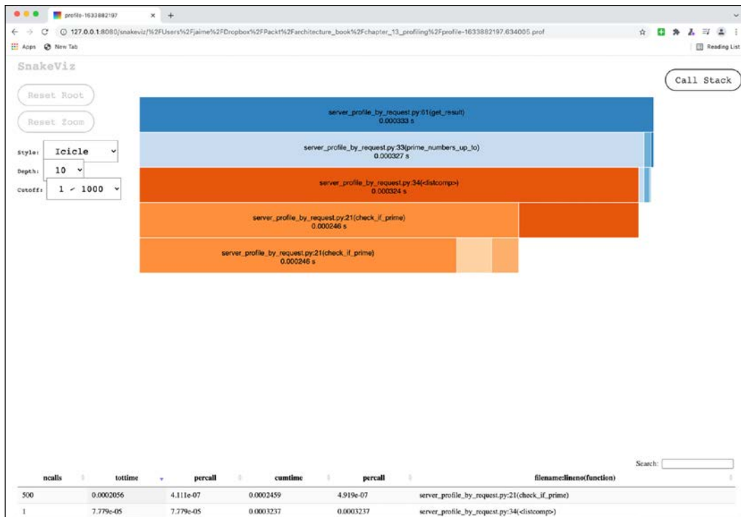
Figure 14.6: The profile information of a single request. The full page is too big to fit here and has been cropped purposefully to show some of the info.
