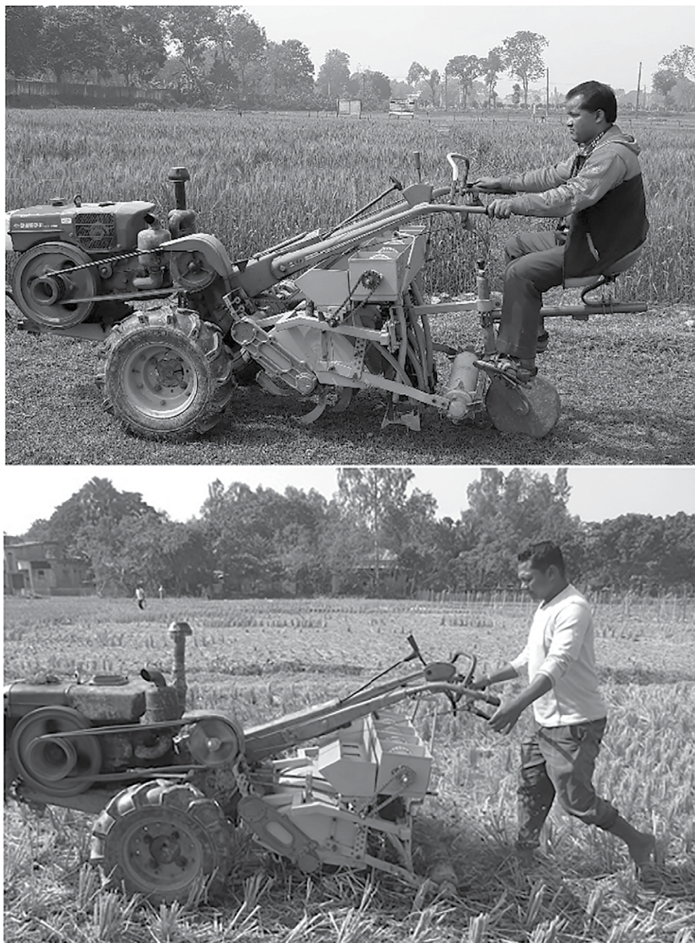
Fig. 28.2. Versatile Multi-crop Planter (VMP) planting in large field and transportation mode (top) and operation mode in smaller plot (bottom) (photos courtesy of Md. Enamul Haque).
