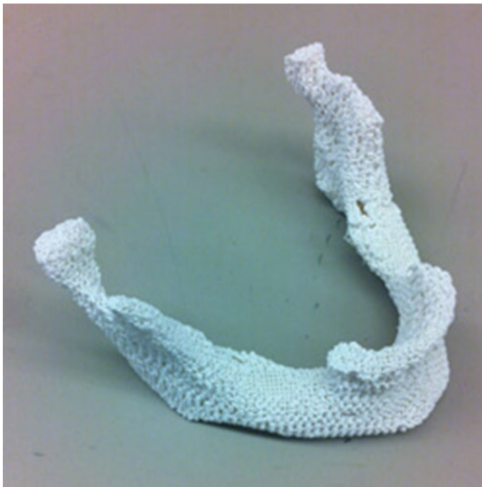
Figure 6.3: 3D-printed scaffold, matching the lower jaw of a female patient [81].
