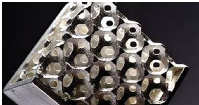
Figure 6.10: Open-cell Al foam by the additive manufacturing [104].
