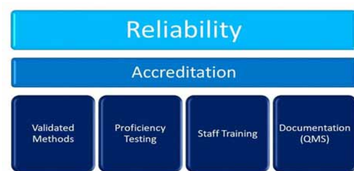
Figure 5. Factors influencing the reliability of a laboratory
