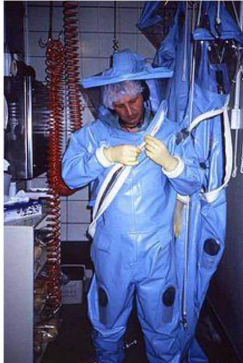
Figure 2. A CDC scientist dons pressurized PPE before entering a high-risk biocontainment lab Source: Wikipedia
