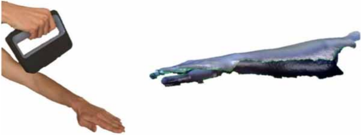
Figure 4. Scanning process of the arm to get the digital model (a) and points cloud (b)
