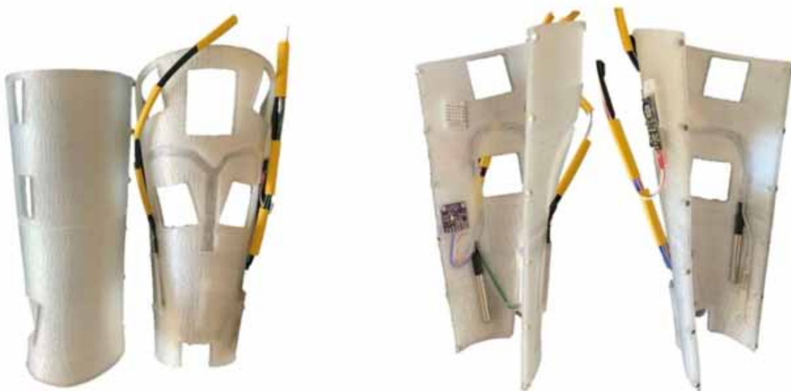
Figure 14. Real leg splint assembled with the sensors (a) and interior view (b)
