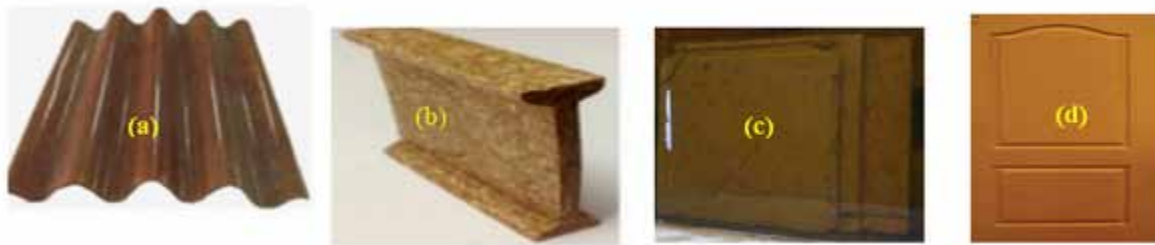
Figure 1. (a) Coir fibre roofing sheet (b) sugarcane waste based panel (c) oil palm waste roofing tiles (d) coir waste door panel (Suoware et al 2020)
