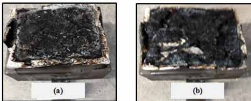
Figure 7. Photographs showing macroscopic images of OPWC and WWC residue surfaces obtained at 50\text{kWm}^2 in the cone calorimeter (a) OPWC (b) WWC
