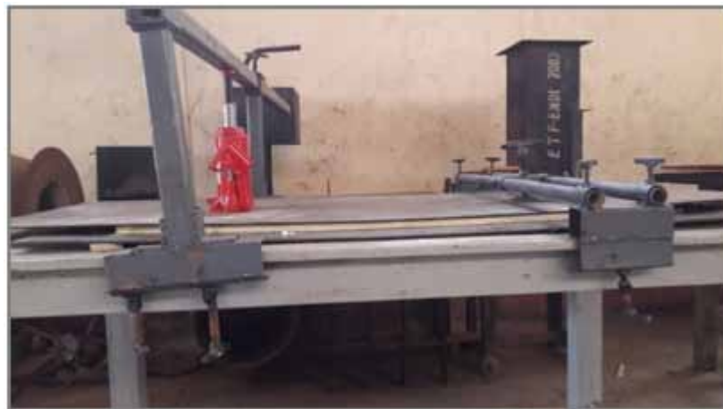
Figure 3. Hand lay-up and compression moulding process of the OPWC and WWC in to different panels of gum Arabic hybridized FR
