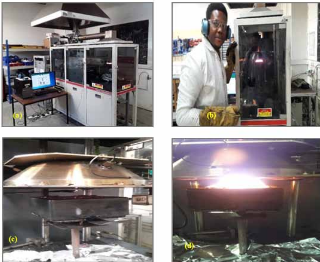
Figure 4. Cone Calorimeter set-up at the Rushbrook Fire laboratory, University of Edinburgh, UK (a) Cone calorimeter apparatus (b) Loading of samples by the researcher (c) ignition process taking place (d) Burning of samples after ignition and data recording
