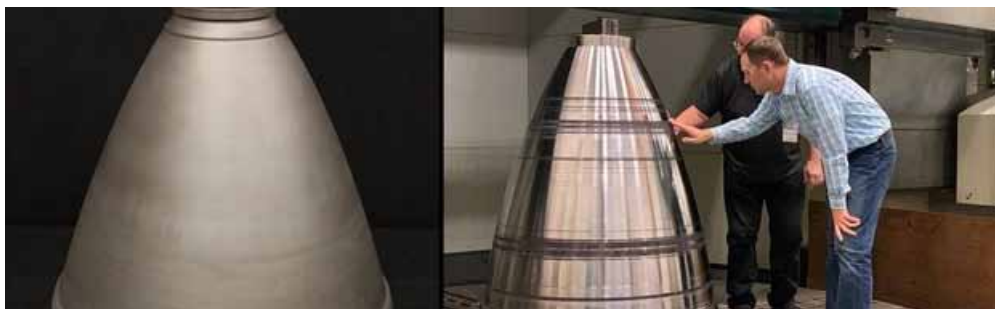
Figure 1. Examples of large scale directed energy deposition integral channel nozzle 1.52 m diameter and 1.78 m height with NASA HR-1 alloy nozzle (Courtesy: NASA)
