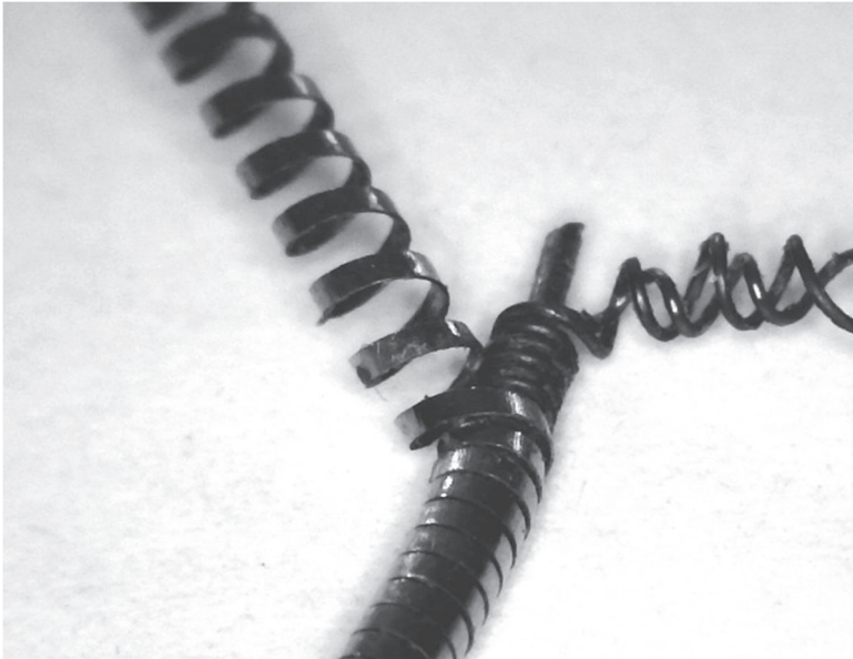
Figure 3.20. Microscopic picture of the several layers of a musical metal string.
