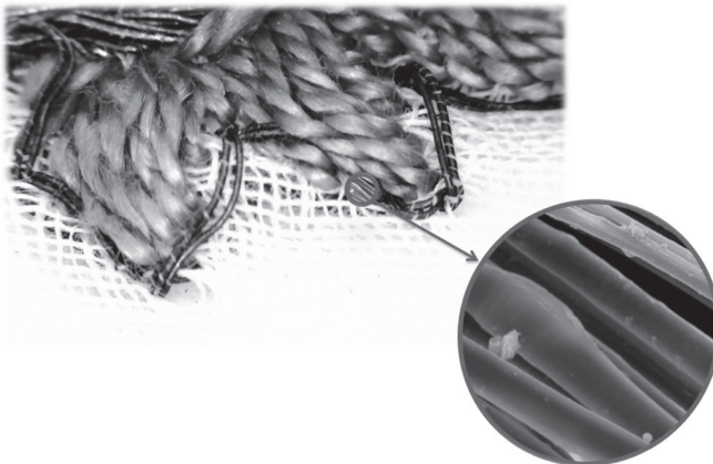
Figure 3.6. Silk fibers detected by SEM microphotography.
