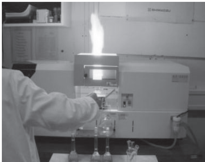
Figure 2.8. Flame absorption spectrometry application for single element analysis of particular elements in the historical samples.
