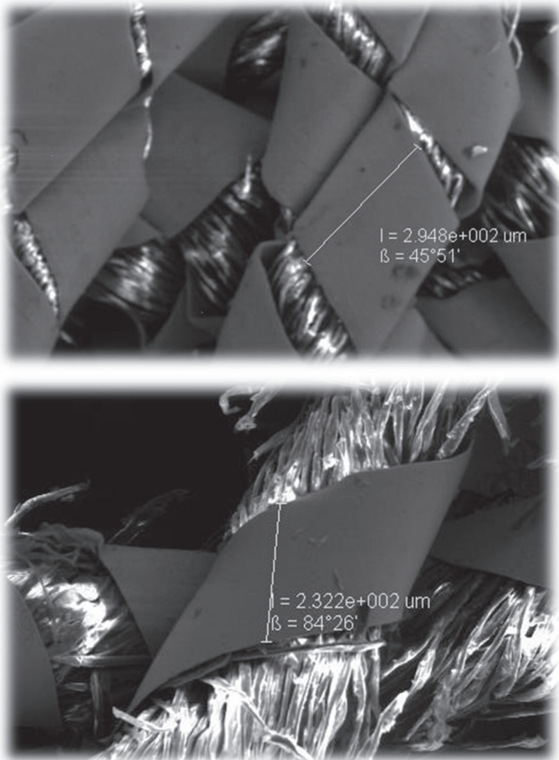
Figure 3.4. Determination of sample size by microphotography. Recorded under 1000× magnification.
