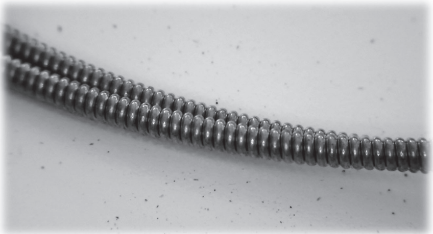
Figure 3.25. Microscopic view of the sample with one material wrapped around its core, 100 \times magnification.
