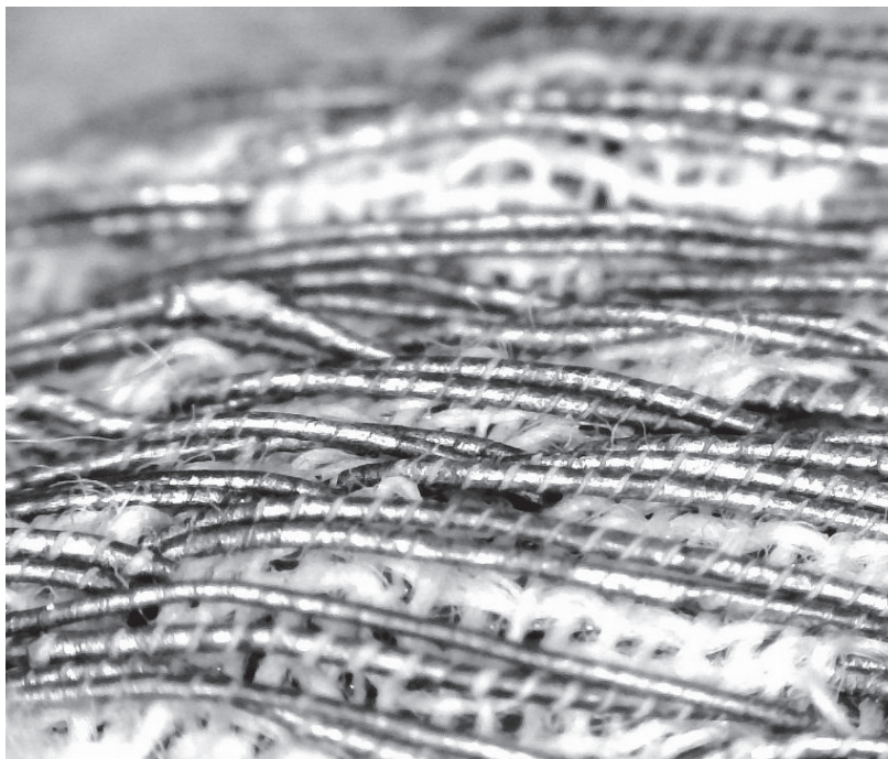
Figure 3.15. Metal threads as a sample for monitoring corrosion processes.
