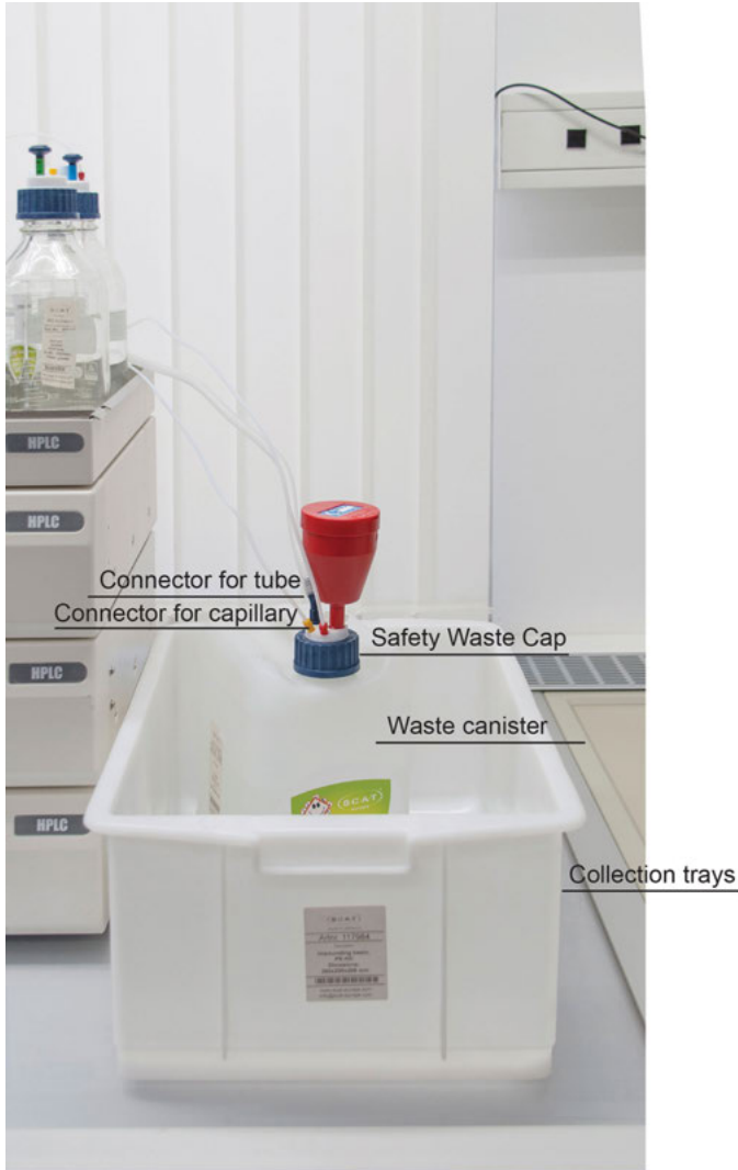
Fig.10.11: Proper HPLC waste collection using a waste canister covered with safety waste cap and stored in secondary containment (collection tray). The canister was properly labeled that contain waste.
