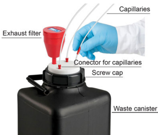
Fig.10.7: Direct collection for effluent of HPLC equipment (three connectors for fitting three capillaries for mobile phase drainage) in closed containers (canister) covered with safety waste cap equipped with exhaust filter. Image source:www.scat-europe.com.
