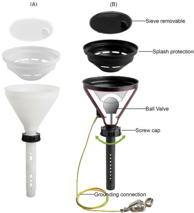
Fig.10.13: Safety funnel with ball valve: (A) general diagram. (B) Illustrative diagram showing the functionality of ball valve in safety funnel. Image source: www.scat-europe.com .
