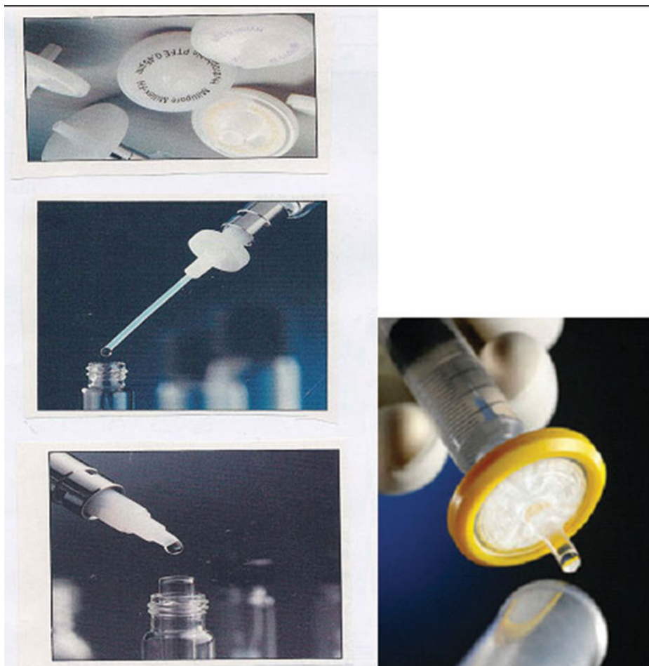
Fig.7.8: Millex-HV syringe filter unit (Millex-HV, pore size = 0.45 \mu\text{m} , hydrophilic polyvinylidene fluoride = PVDF) for clarification of aqueous and mild organic solution before injection in HPLC (Merck).
