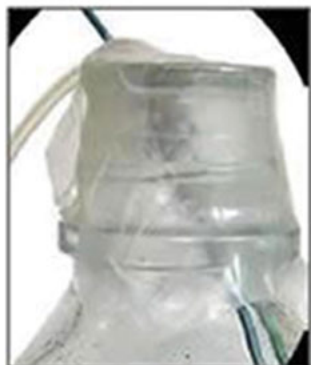
Fig.10.6: Improper HPLC mobile phase reservoir covering practices. (A) Cover with aluminum foil and (B) cover with parafilm.
