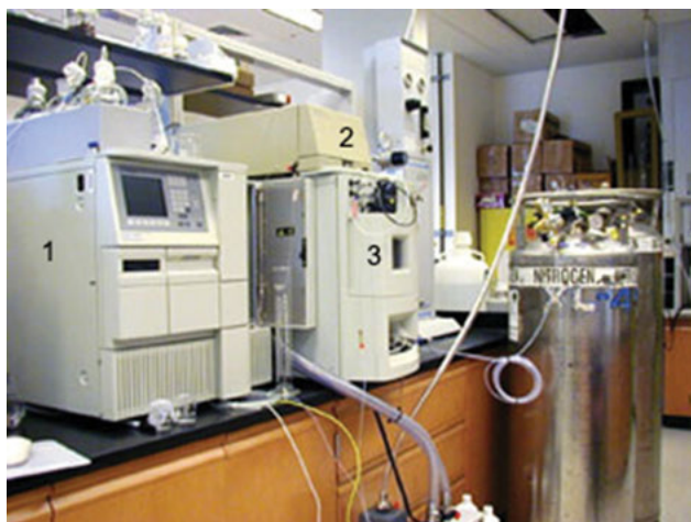
Fig.9.4: Configuration showing a combination of Waters HPLC system (Waters Alliance 2695 Separation Module) (1), photodiode diode array detector (Waters 996) (2) and Waters – micromass ZQ detector (3). Reproduced with permission from Waters Corporation ( www.waters.com ) [16].
