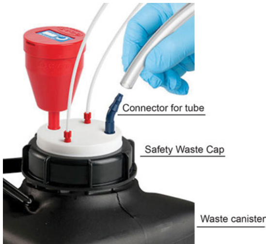
Fig.10.10: Safety waste cap ready for connection and fits two capillaries with an outer diameter of 2.3 and 3.2 mm for mobile phase drainage, one tube (the standard connector design is for flexible tubes with 6.4–9.0 mm inner diameter) and exhaust filter.
