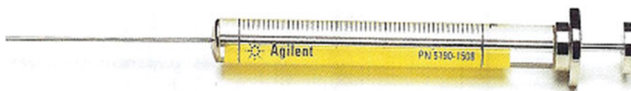
Fig.4.6: Manual syringe for injecting the sample manually in the HPLC injection valve which is fitted in the plunger.
