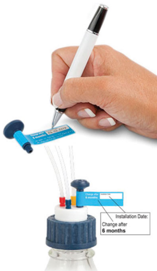
Fig.10.4: Change advice label on air valve. Image source: www.scatt-europe.com.
