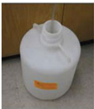
Fig.10.12: Improper HPLC waste collection practices using open bottle, unlabeled and the bottle not found in secondary containment.
