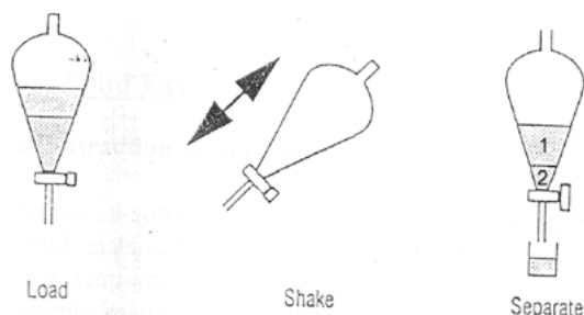
Fig.7.2: A separator funnel for LLE which depends on the density of the immiscible organic solvent. It will separate after shaking either to the upper (1) or lower (2) phase.
