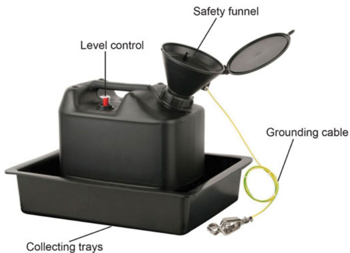
Fig.10.18: Disposal unit for collection of HPLC solvent waste. Image source: www.scat-europe.com.
