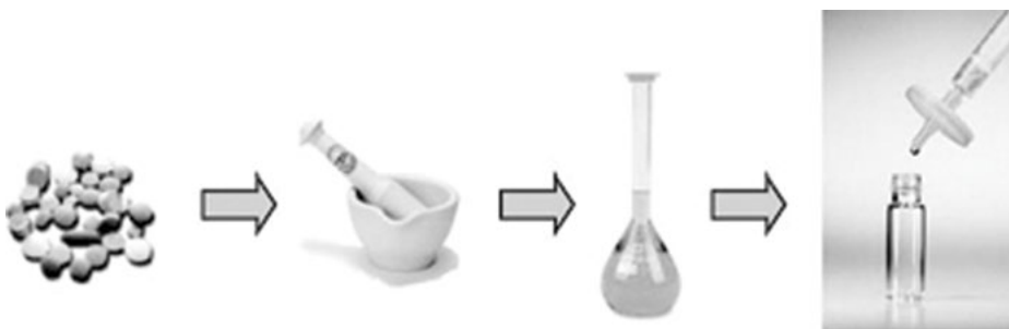
Fig.7.7: The common sequence of sample preparation steps for solid drug products: grinding, extraction, dilution and finally filtration.
