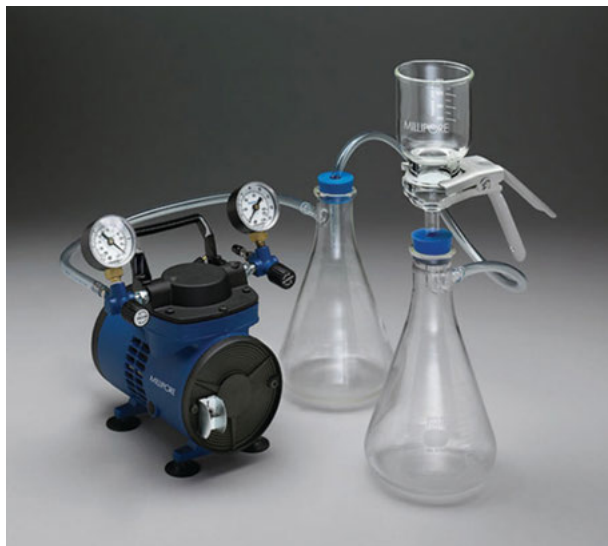
Fig.3.7: The Millipore conventional vacuum filtration and degassing system. Reprinted with permission from Millipore Co., Waters Chromatography Division, 43 Maple Street, Milford, MA 01757, USA [22].
