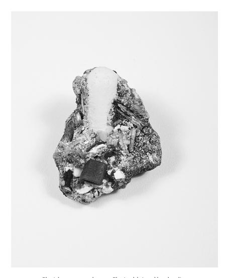
FIGURE 2.2. Plastiglomerate sample, 2013. Plastics debris and beach sediment, including sand, wood, rock, and shell debris. Photo: Jeff Elstone, courtesy of Kelly Jazvac.
